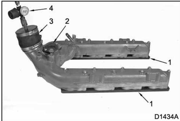
**Figure 105 Set up for intake manifold pressure test**
