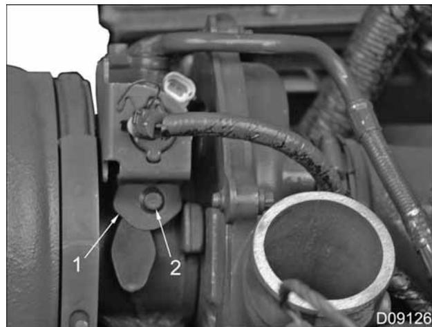
**Figure 78 Retaining bolt for VGT Control valve**
