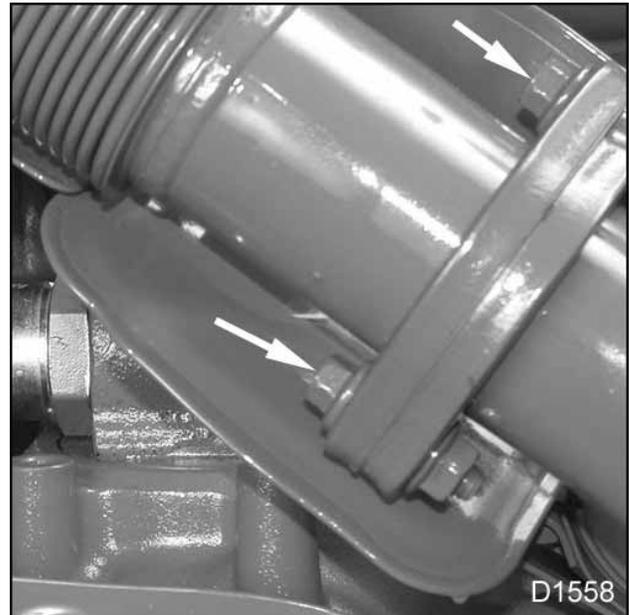
**Figure 84** Exhaust tube bolts (upper right)
