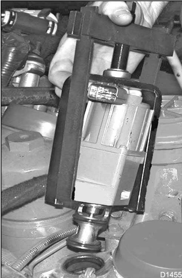
**Figure 94 EGR valve removed**
