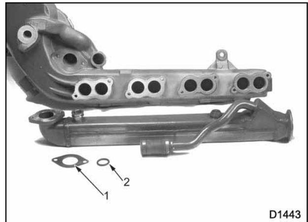
**Figure 102 EGR cooler assembly**
