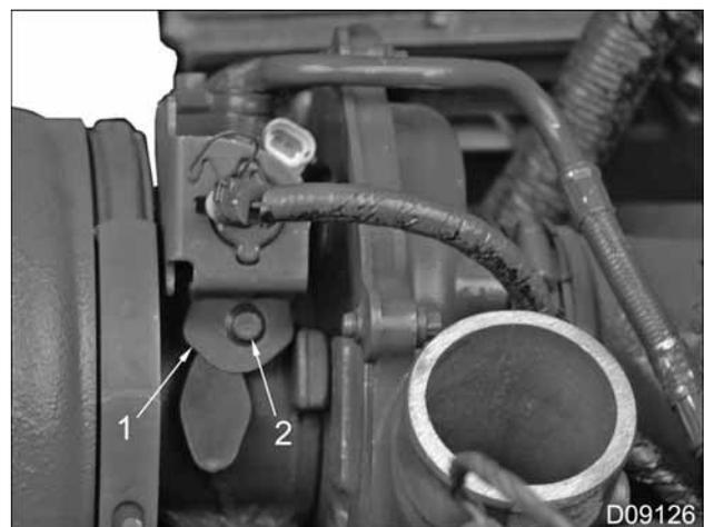
**Figure 47** Retaining bolt for VGT control valve
