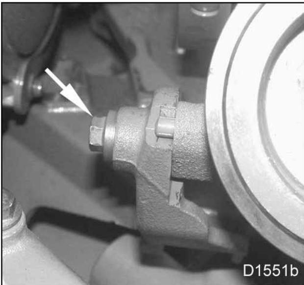
**Figure 55 Center mounting bolt and spacer for VGT**
