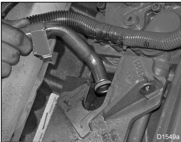
**Figure 59 Removal of oil drain tube for VGT**
