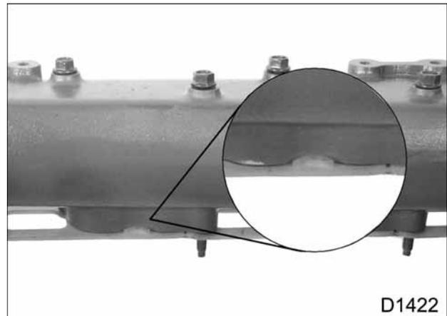
Figure 113 Intake manifold gasket with centering tab
