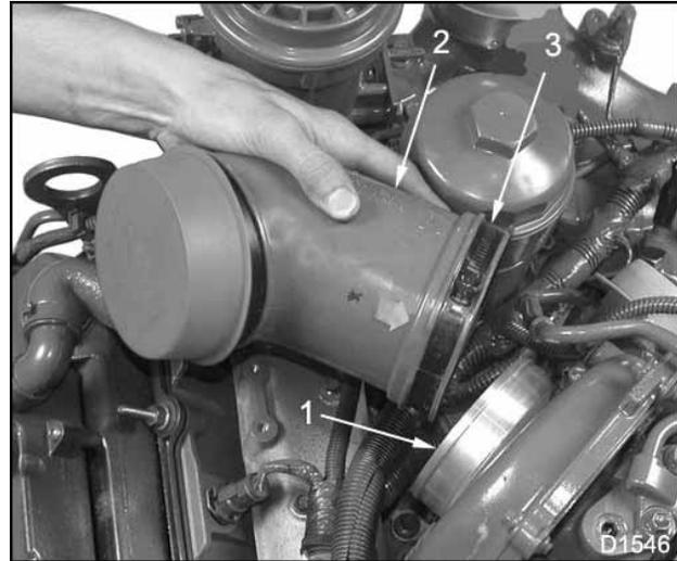
**Figure 50 Air inlet duct**
