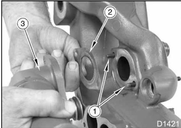
**Figure 107 EGR cooler connection to intake manifold**
