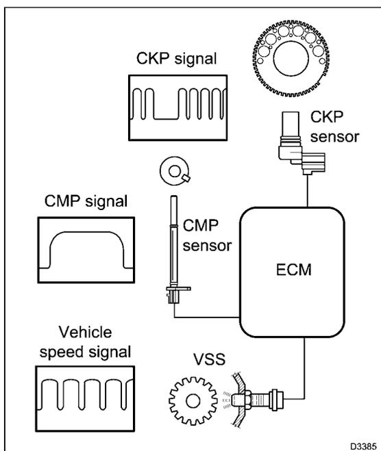
Figure 37 Magnetic pickups
