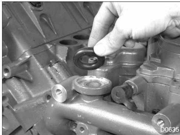
Figure 112 Front module seal
