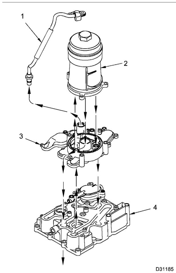
**Figure 29 Oil cooler base and oil filter base**
