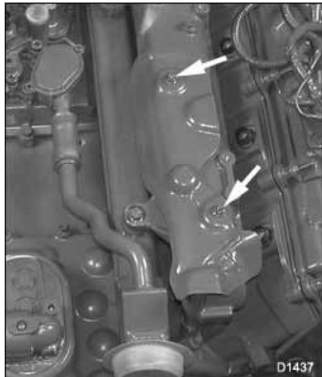
**Figure 95 Intake heat shield mounting nuts (right side)**
