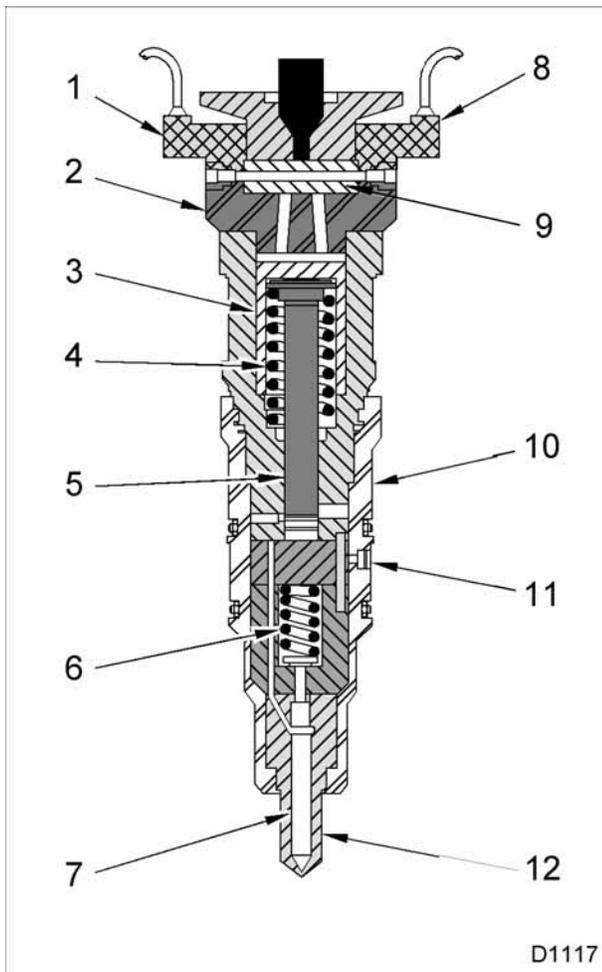
**Figure 24 Fuel Injector**
