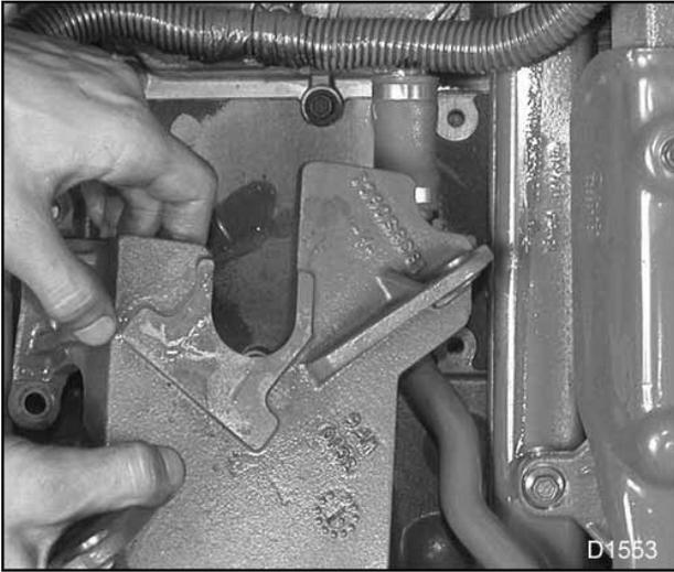
21. Lift up the left side of the bracket first so the right side can clear the EGR cooler coolant inlet tube.
