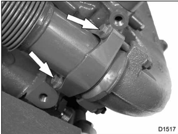
**Figure 122** Mounting bolts for right exhaust tube
