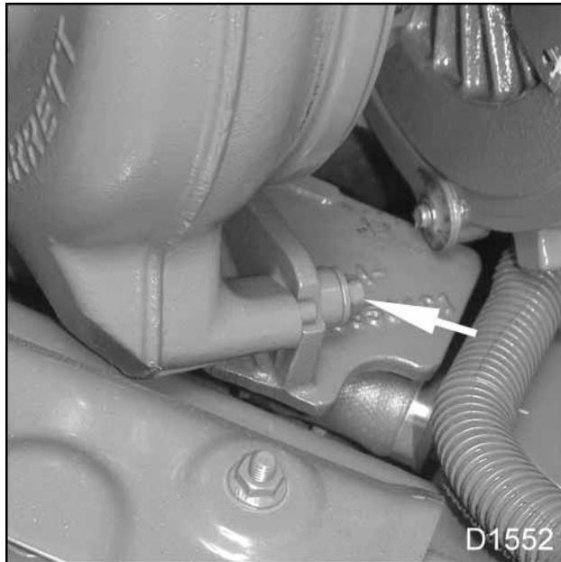
**Figure 57 Front mounting bolt and spacer for VGT**
