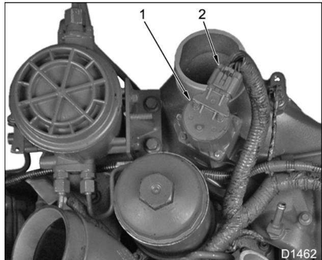
**Figure 89** EGR valve and 8-pin electrical connector
