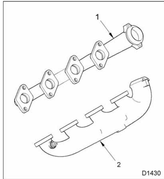
**Figure 82 Exhaust manifolds**
