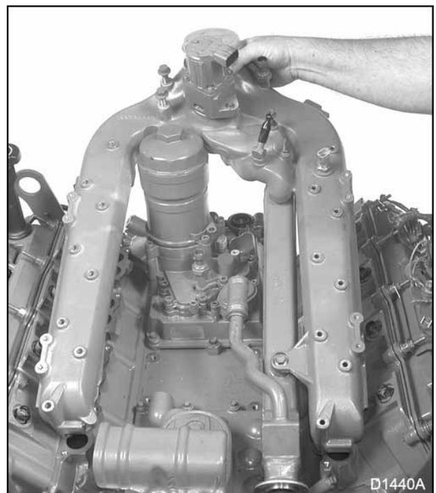
Figure 114 Intake manifold and EGR cooler assembly
