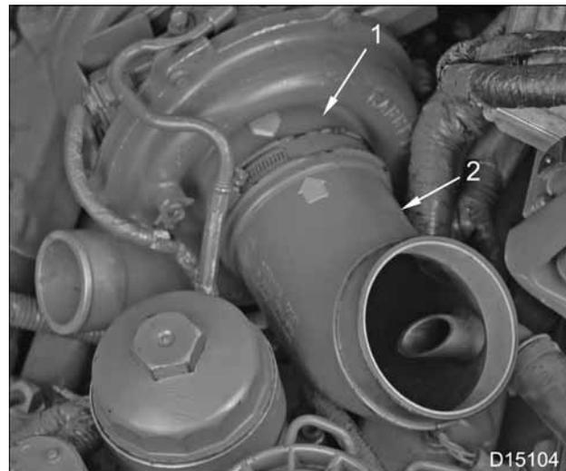
**Figure 74 Air inlet duct to VGT**
