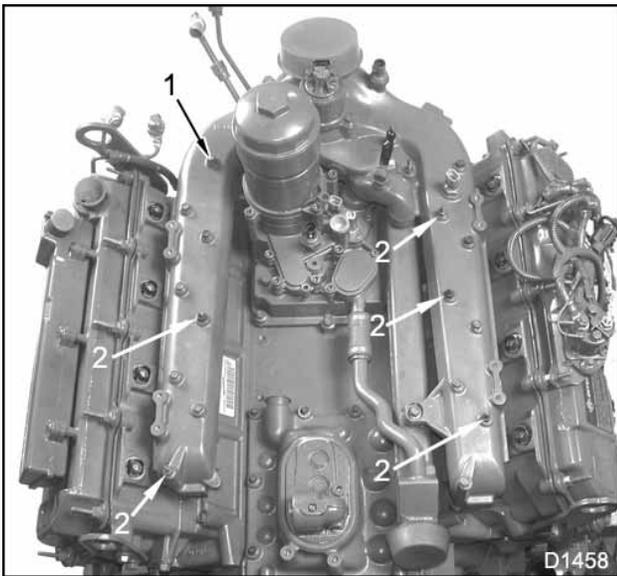
**Figure 115 Dog point bolts and stud bolts**
