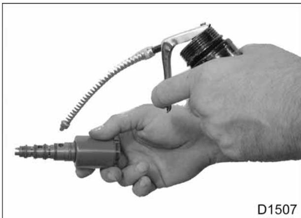
**Figure 76 O-ring lubrication**
