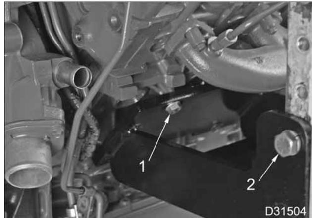
**Figure 44 Mounting bolts for Engine Stand Mounting Bracket**
