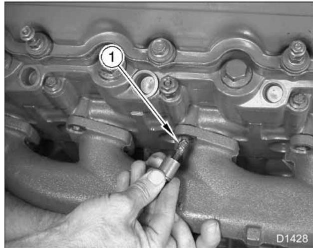
**Figure 124** Bolt and spacer for left exhaust manifold
