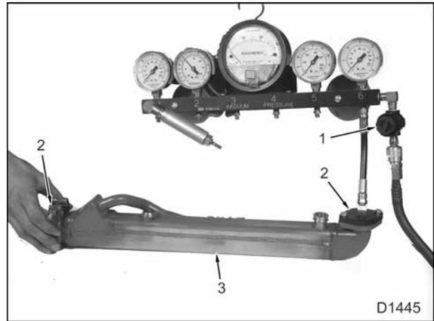
**Figure 106 EGR cooler with pressure test plates installed**
