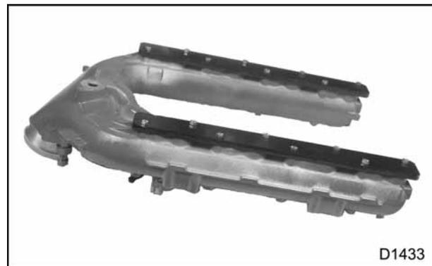
**Figure 104 Test plates installed on intake manifold**
