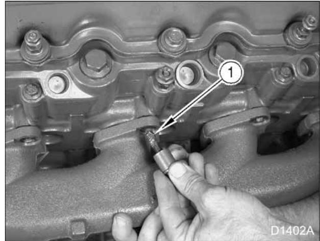
**Figure 120 Right exhaust manifold bolt and spacer**
