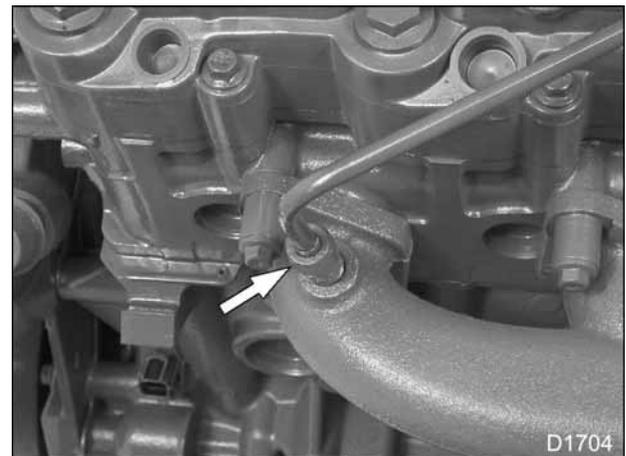
**Figure 85** Tube fitting for EBP sensor
