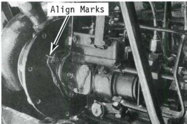
Fig. 114—On four-cylinder engines, injection pump is properly timed to engine when marks on pump flange and engine front plate are aligned.
