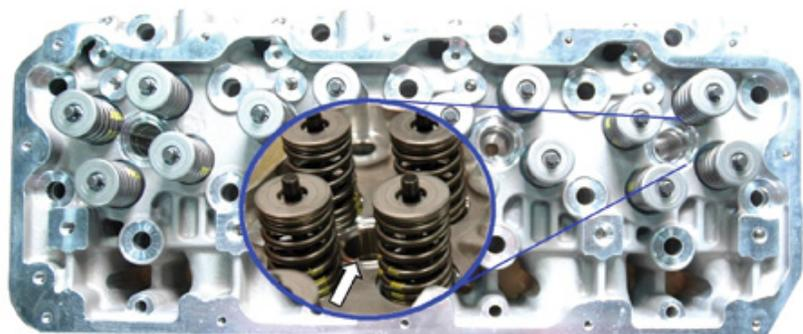
**Figure 7.** The early cylinder head through mid '04 MY had injectors under the valve cover and the injector sealed deep in the head as seen in the inset with arrow.
