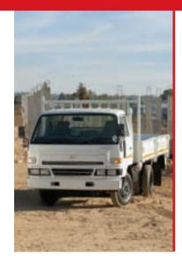
Tare and gross allowable mass are the determining factors. When evaluating a truck, examine its payload efficiency. A measure of payload efficiency is to strive for the optimum payload GVM ratio. Rigid vehicles: >55 % to 60 % of GVM \* Articulated: >60% of GCM.
