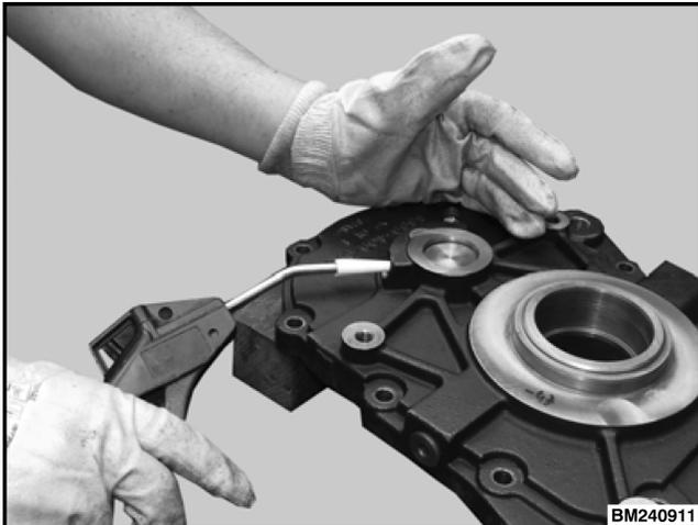
**Figure 15. Removing the Cap**
