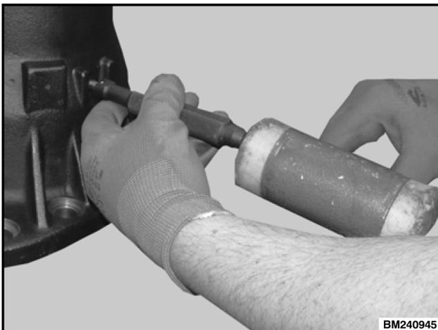
**Figure 10. Installing the Breather**
