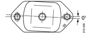
*Upper and lower parts of the insulators should be parallel longitudinally.*
