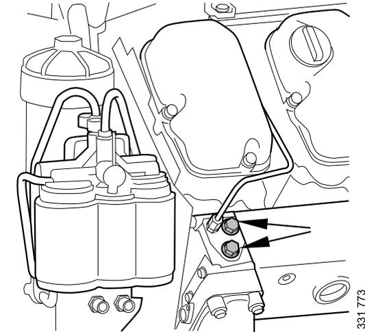
Connection of sensor for coolant temperature, G1/2". If necessary, an adapter can be ordered as extra equipment
