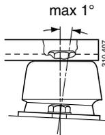
*The engine bracket and frame or engine bed should be parallel.*
