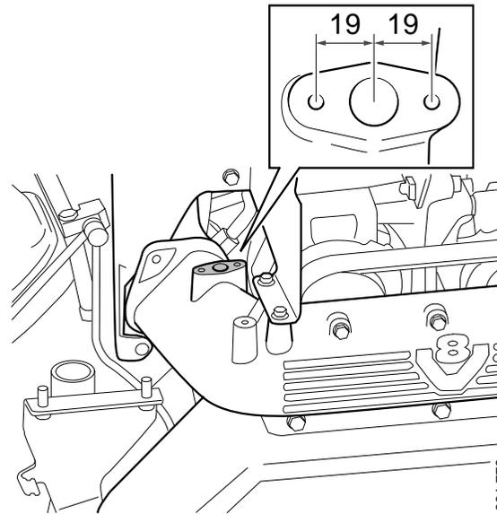
Connection of sensor for charge air pressure and charge air temperature, Ø 16 mm, 2 x M6 screws
