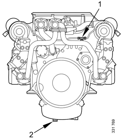
1. Connection of oil pressure sensor. The three-way union must be renewed for a four-way union, which can be ordered as extra equipment
