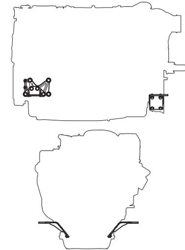
*Examples of rigid engine suspension*
