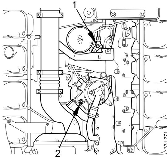
1. Connection of sensor for fuel pressure, M10x1
