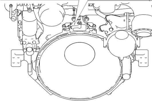
Connection of sensor for coolant temperature and coolant pressure
