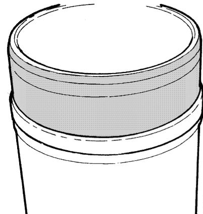
*Lubricate the lower part of the cylinder liner before fitting it in place.*
