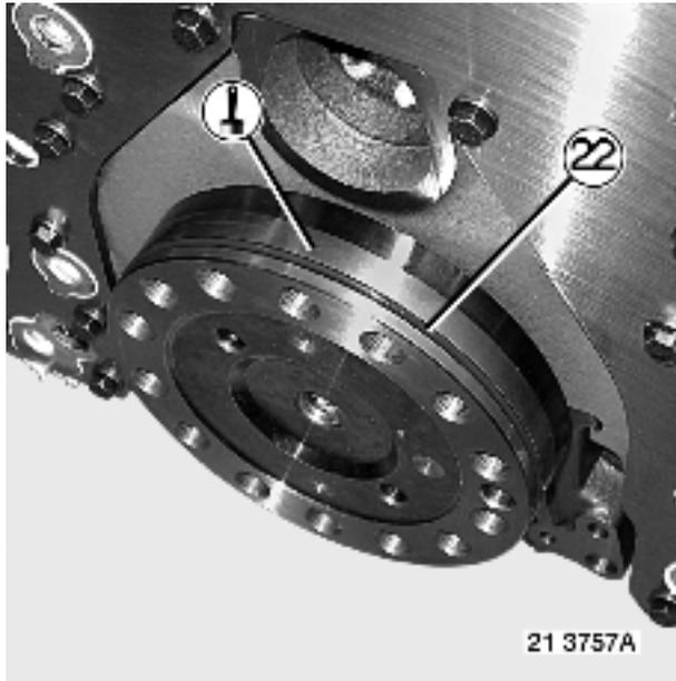
Lightly oil a new O-ring **(22)** and install.
