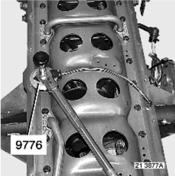
Tighten bolts (1) to torque.
