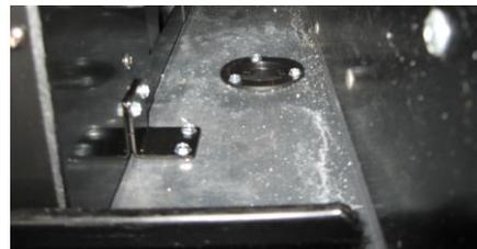
*Failure to use the proper cable loom and/or grommet will result in damage to cables, unit and/or vehicle. Always seal all open areas in grommet with silicone when installation is complete. Silicone is not provided in kit.*
