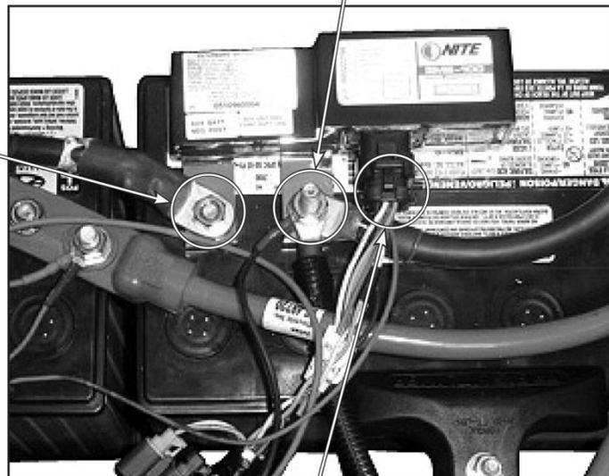
1. Attach connector from NITE system wiring harness to BMS-100 mating connector.
