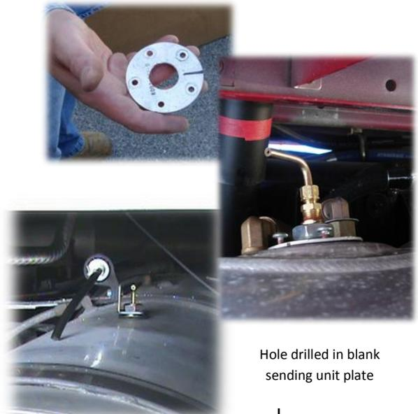
Hole drilled in tank
