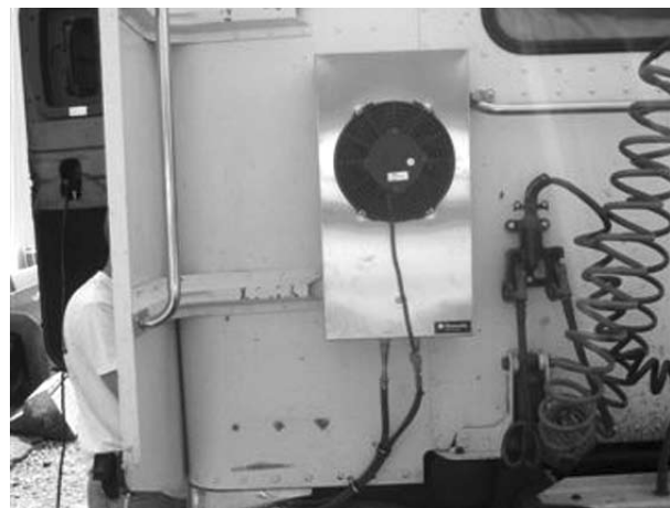
Figure 2b - Condensing unit mounted on back of sleeper
