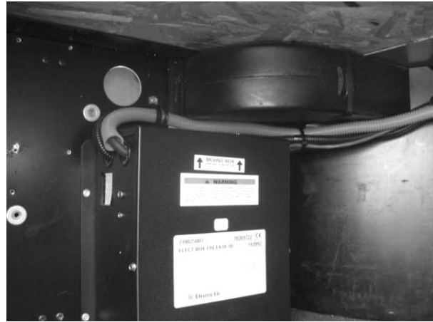
Figure 4 - Possible PLB mounting location
