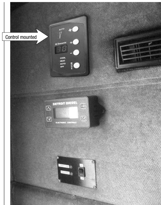
Figure 3a - Control/Display panel mounted
