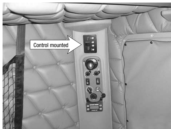
Figure 3b - Alternative Control/Display panel mounting location
