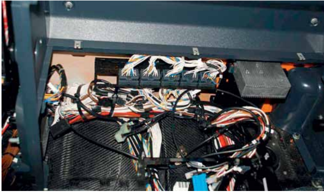
Coding adapter under rear stowage box
