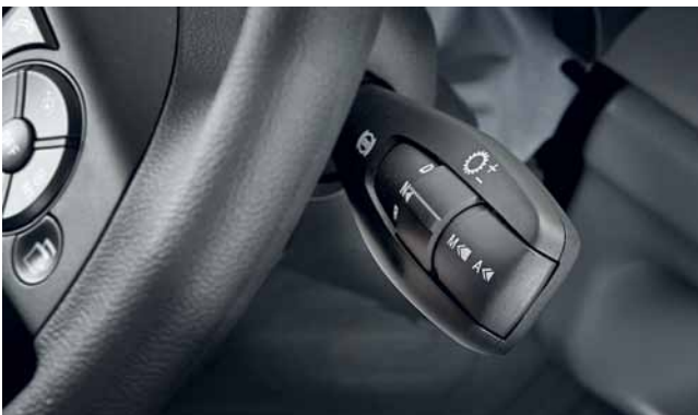
Telligent® engine management multifunction control lever
