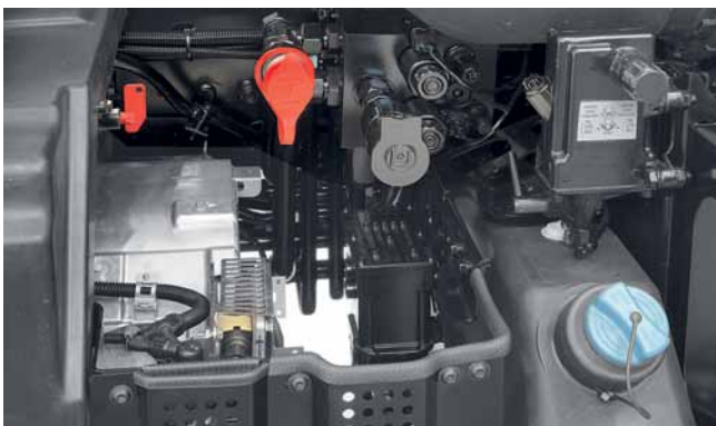
Circuit 2 hydraulic valve block
