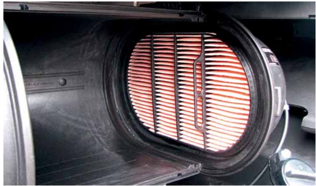
Safety insert in air filter housing
