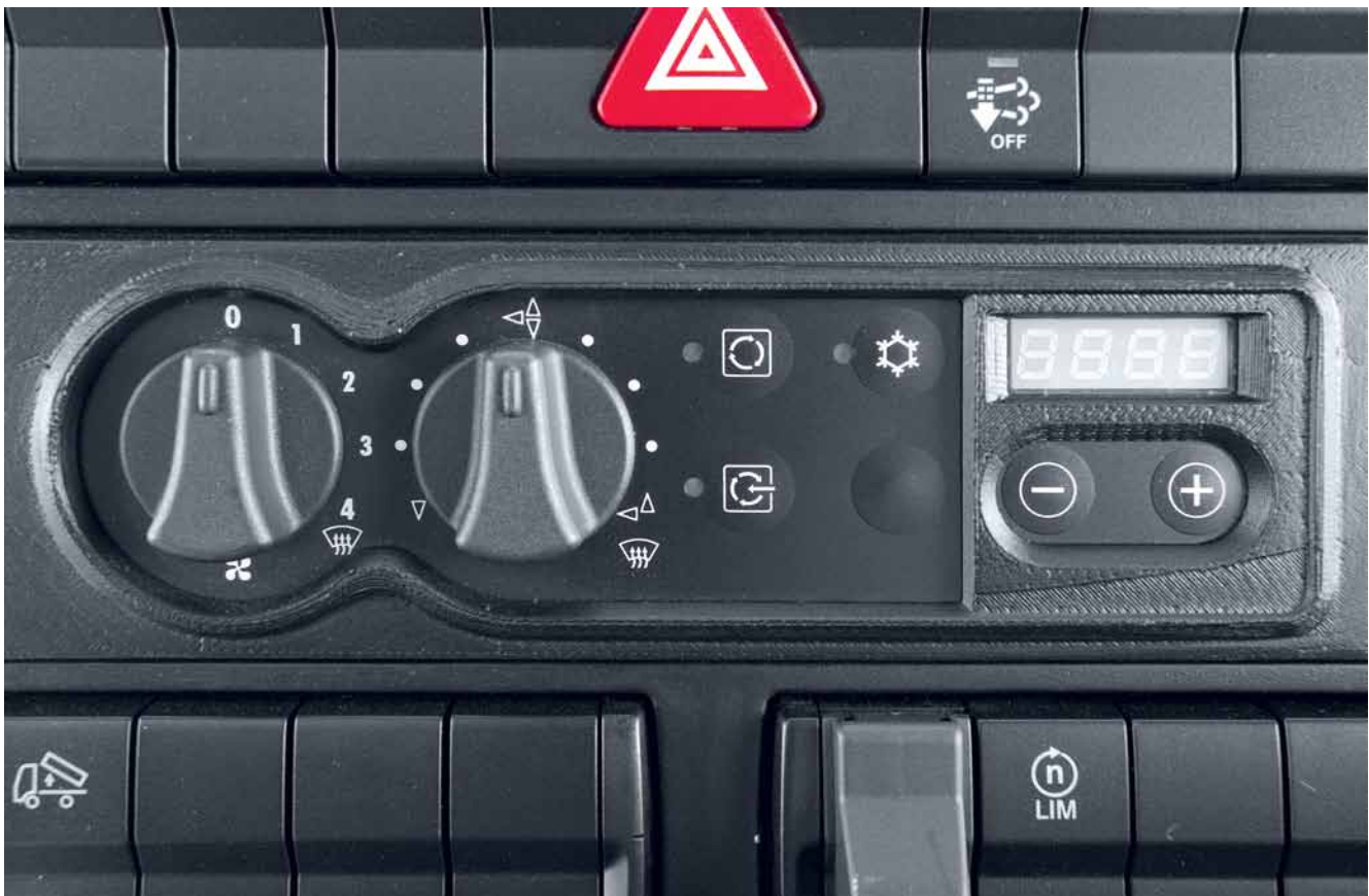
Air conditioning system (D6F)
