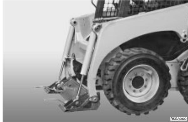
1 - Remove the pin (1) and fully retract the piston rod (2).
