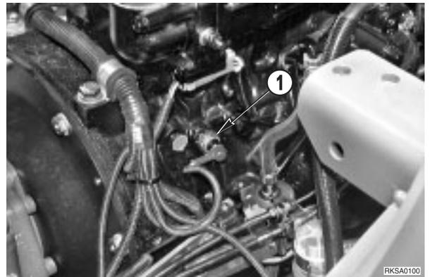
3 - Mount the adapter **D1** and connect the pressure gauge **D2**.
