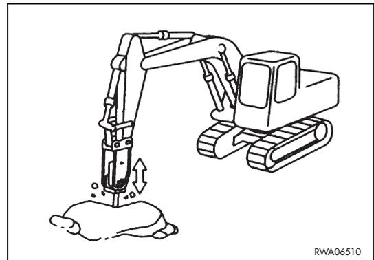
7 - Lifting the machine by levering on the hammer bit with the bucket cylinder extended to the end of its stroke.
