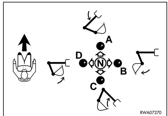
If the levers are operated in directions that are inclined with respect to the machine axis, simultaneous movements proportional to the angle of inclination are obtained, since the two hydraulic distributors corresponding to each single function are engaged at the same time.
