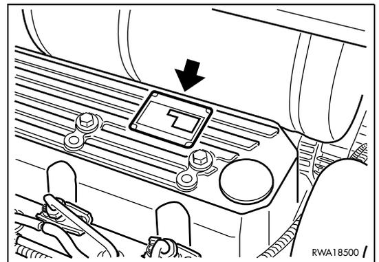
The exhaust gas emission plate is applied to the front side of the tappet cover.
