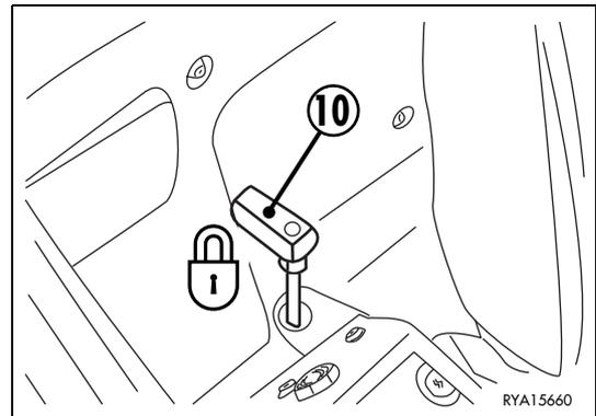
When the lever (10) is in the lock position, it prevents the rotation of the upper structure.
