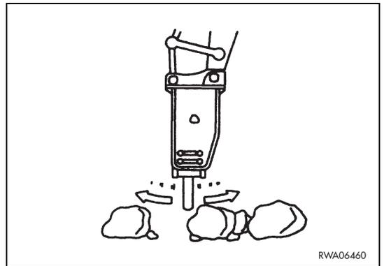
2 - Rotating the upper structure while using the hammer.
