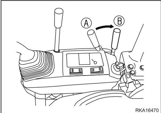
2. Set the safety lever (2) to the “free” position and raise the bucket from the ground.
