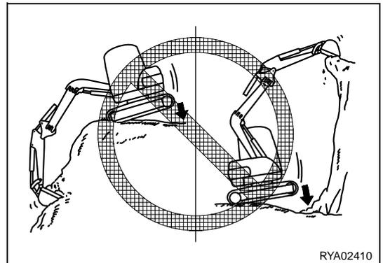
● **SUPPORT THE MACHINE WITH BOTH SIDES OF THE BLADE**
