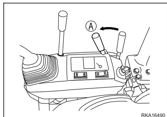
3. Lower the bucket keeping it in horizontal position, until its bottom touches the ground.
