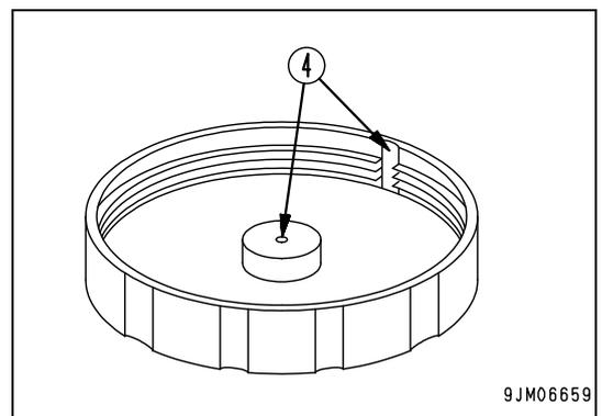
**CHECKING THE OIL LEVEL IN THE HYDRAULIC TANK AND TOPPING UP**
