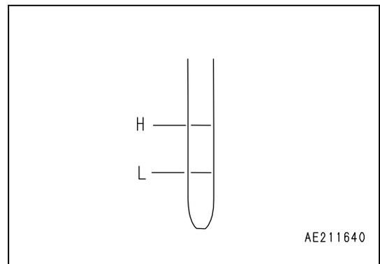
5. If the oil level is above the H mark, drain the excess oil through the drain plug (P), and check the oil level again.
