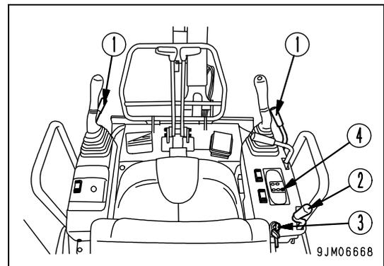
1. Make sure that the safety lever (1) is in the “locked” position (L). If the safety lever is in the “free” position (F), the engine cannot be started.
