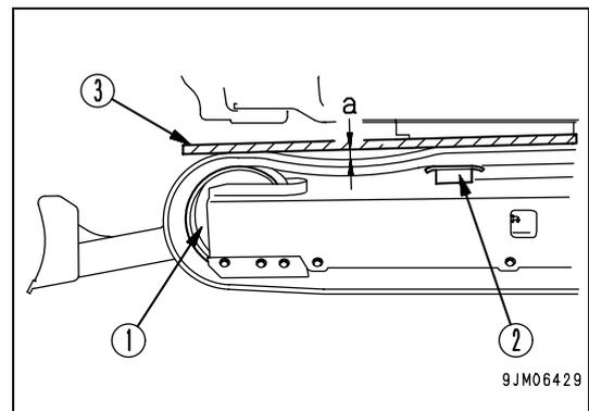
If the track tension does not correspond to the standard value, adjust it by proceeding as indicated below.
