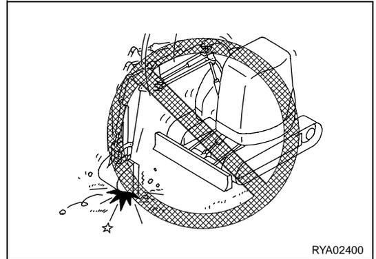
● **OPERATIONS FOR WHICH IT IS NOT ALLOWED TO EXPLOIT THE FORCE OF GRAVITY OF THE MACHINE**
