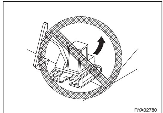
3. Do not proceed along the edges of a slope or on uneven ground keeping one track in horizontal position and the other inclined or partially raised (with machine inclination exceeding 10°C). To avoid damaging the rubber tracks, always proceed with both tracks resting on the same horizontal plane.
