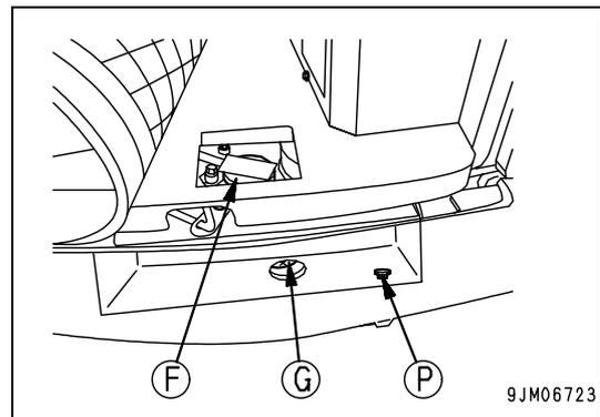
3. If the oil does not reach the level (L), lift the mat (1), remove the cover (2) and the cover on the filler neck (F), then top up through the filler neck (F) using the oil recommended in the lubricant chart (see "4.4 FUEL, COOLANT AND LUBRICANTS").
