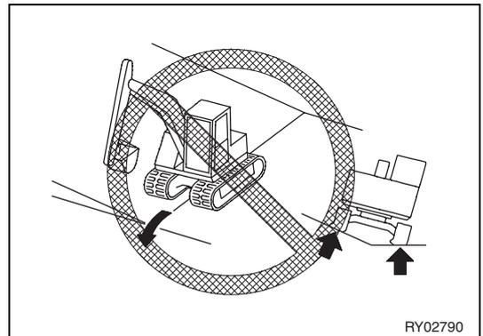
4. If the machine is operated in the conditions described in points from 1 to 3 above, do not change direction if the tracks do not adhere perfectly to the ground, see figure.
