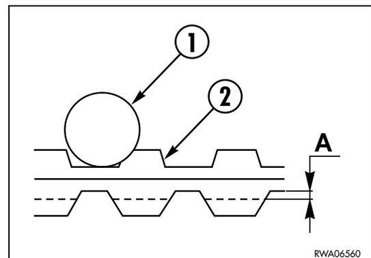
2. When the steel core is visible in two or more points of the track.
