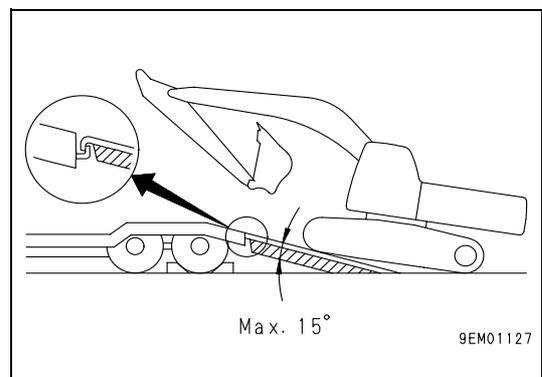
During the loading and unloading operations, always use ramps or a platform and proceed as indicated below.
