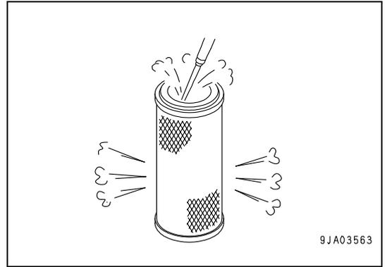
6. After the cleaning operations, inspect the filtering surface for damage by introducing a lamp into it and carefully check the front gaskets. If the cartridge is damaged, change it.
