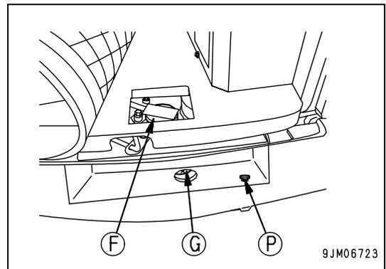
14. Extend the boom, arm and bucket cylinders completely, as shown in the figure, and remove the filler cap (F). Put back the cap and pressurize the tank by lowering the equipment to the ground.
