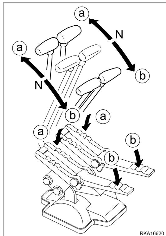
7. Boom swing control pedal locking device
