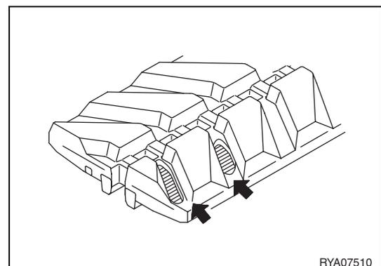
3. When more than half of the steel core cords at the centre of the track are cut.
