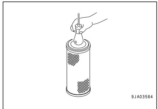
7. Remove the cloth or adhesive tape used to cover the air connector inside the filter body.
