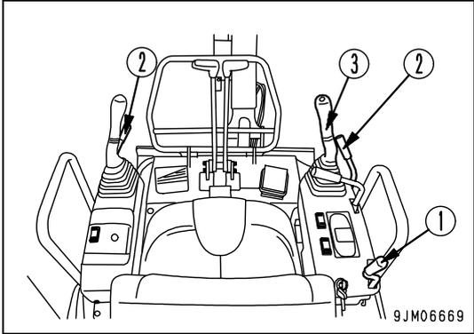
1. Shift the accelerator lever (1) from the idling (A) to the intermediate speed position (B), and let the engine idle at medium speed for at least 5 minutes.
