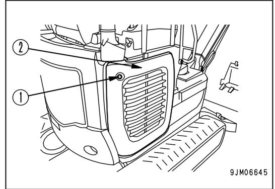
2. Pull the radiator cover (2) and open it completely. The cover (2) is kept open by the apposite rod (3).
