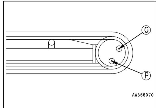
Carry out some forward and backward movements, stop the machine and check the levels again. Always use oil of the prescribed type (see "4.4 FUEL, COOLANT AND LUBRICANTS").
