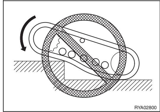
6. Furthermore, if the machine travels in reverse, a gap forms between the carrier roller, the idler roller, and the rubber track.
