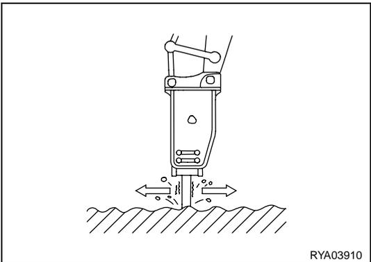
4. Working with the breaker in horizontal position or even more inclined.
