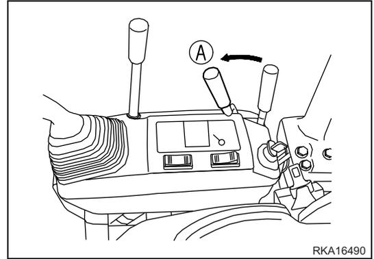
8. Lift the work equipment, make sure that the travel direction is in line with the ramps and start travelling slowly. Lower the work equipment as much as possible, without causing interferences. When the machine is on the ramps, do not use any control lever apart from the travel levers.
