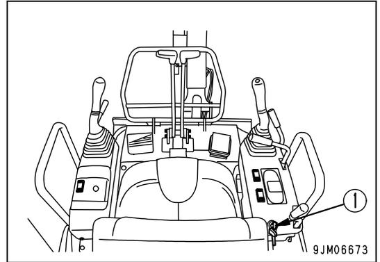
2. Turn the ignition key (1) to position OFF to stop the engine.
