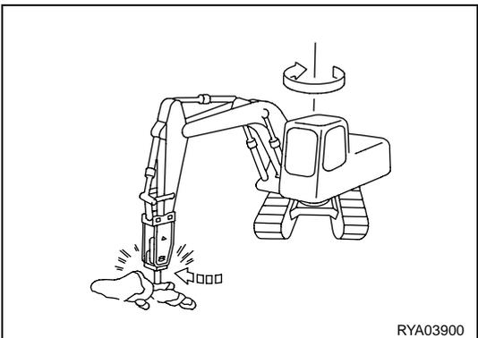
3. Moving the tool while it is hitting the material to be broken.
