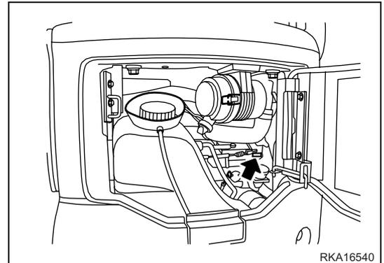
The exhaust gas emission plate is applied to the counterweight.
