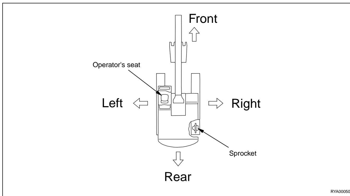
In this manual, the terms front/forward, rear/backward, left, and right refer to the travel direction as seen from the operator seat when it is facing the front and the sprocket is at the rear of the machine.
