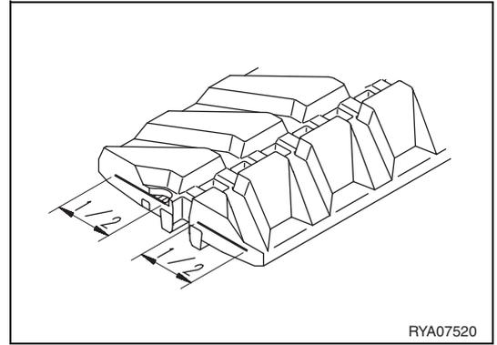
4. When one or more steel cores have come off the track or are pushed out due to excessive tension.
