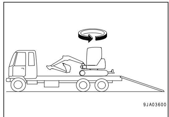
**SECURING THE MACHINE ON THE MEANS OF TRANSPORT**
