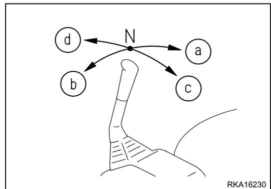
The control lever (3) is positioned on the operator's right and controls the boom and the bucket.
