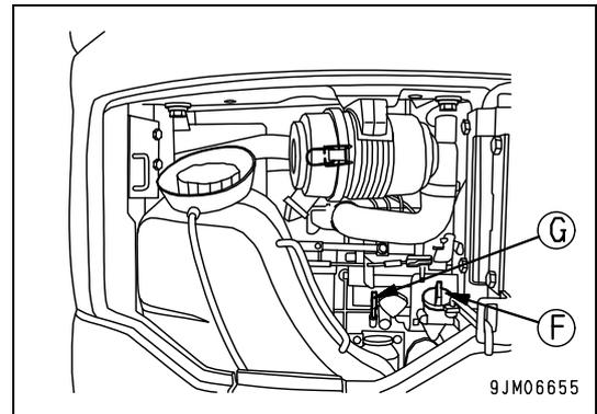
4. The oil level must be included between the H and L marks; if the level is near the L mark, top up through the filler neck (F), using oil suitable for the ambient temperature, as indicated in the lubricant chart (see "4.4 FUEL, COOLANT AND LUBRICANTS").
