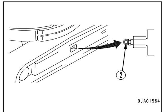
2. When after the injection of grease the idler roller sliding plate reaches the measure «S» of 0 mm and the track is not sufficiently stretched, this means that the pins and bushings are excessively worn. Therefore, it is necessary to exchange or replace the pins and bushings.
