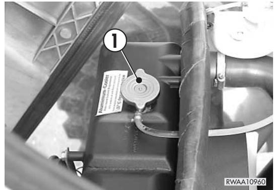
The radiator cap can be reached after opening the engine hood (See “3.5.1 ENGINE HOOD”).
