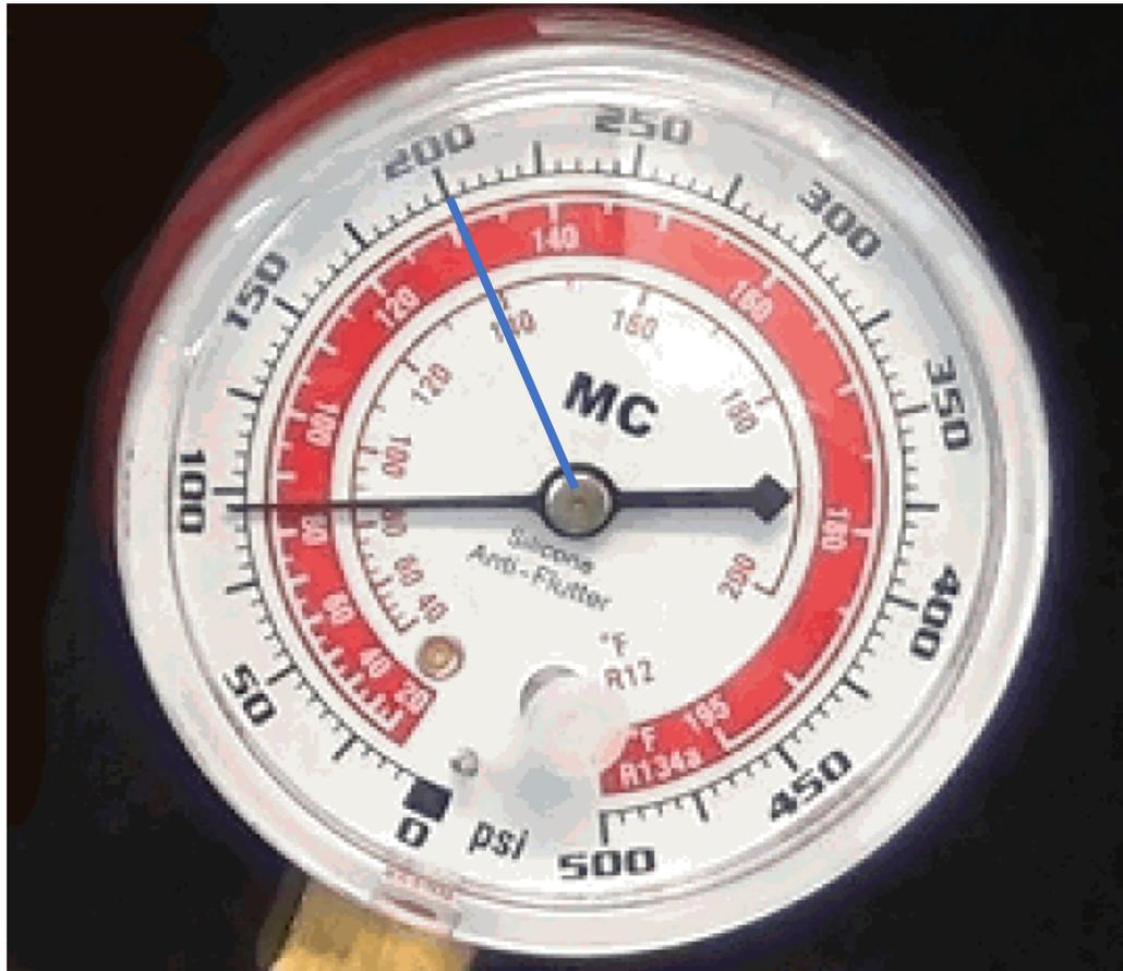
Many refrigerant gauge sets have an inner scale that reads the saturation (boiling) point of the refrigerant.
