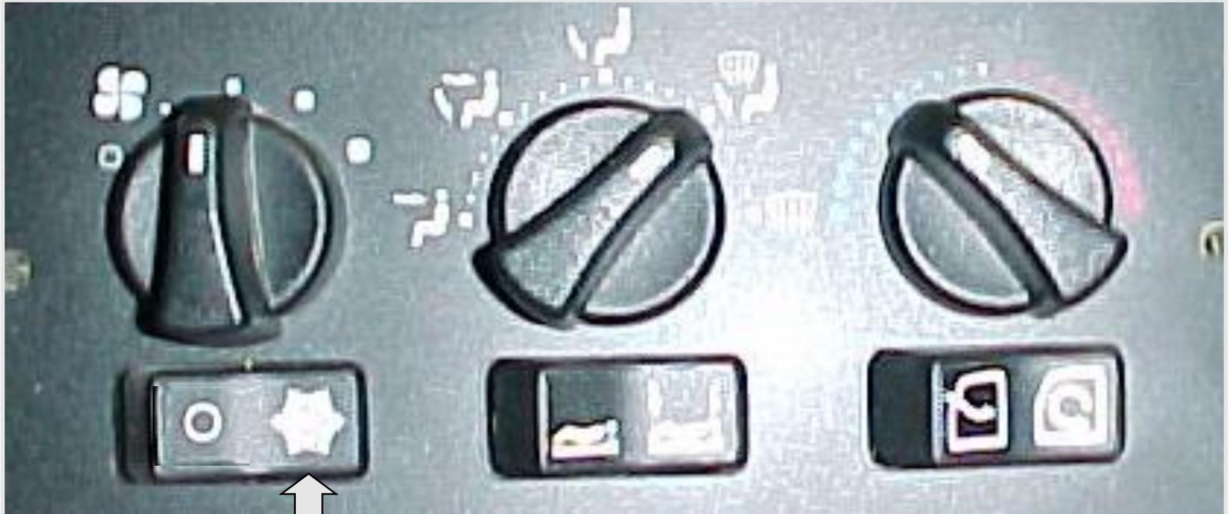
A/C switch on the left side of the control panel
