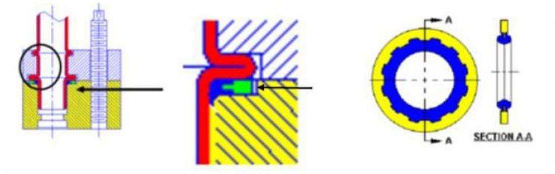
***Per Parker Engineering (manufacturer of the seals), these are not to be lubricated during installation.***
