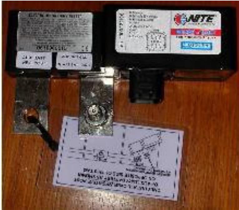
This device monitors the auxiliary batteries for state of charge, communicates with the KIM system and controls the battery separator solenoid.
