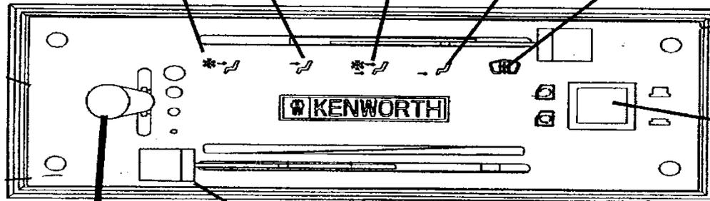
**BLOWER SWITCH:** FOUR POSITIONS: OFF, LOW, MEDIUM, AND HIGH. MUST BE ON FOR THE A/C SYSTEM TO WORK.
