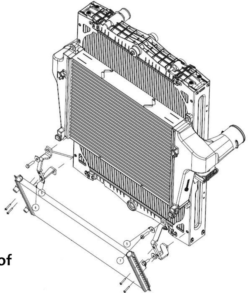
**Note: Due to the low mount design of the condenser, road debris buildup inspection is an initial diagnostic step**
