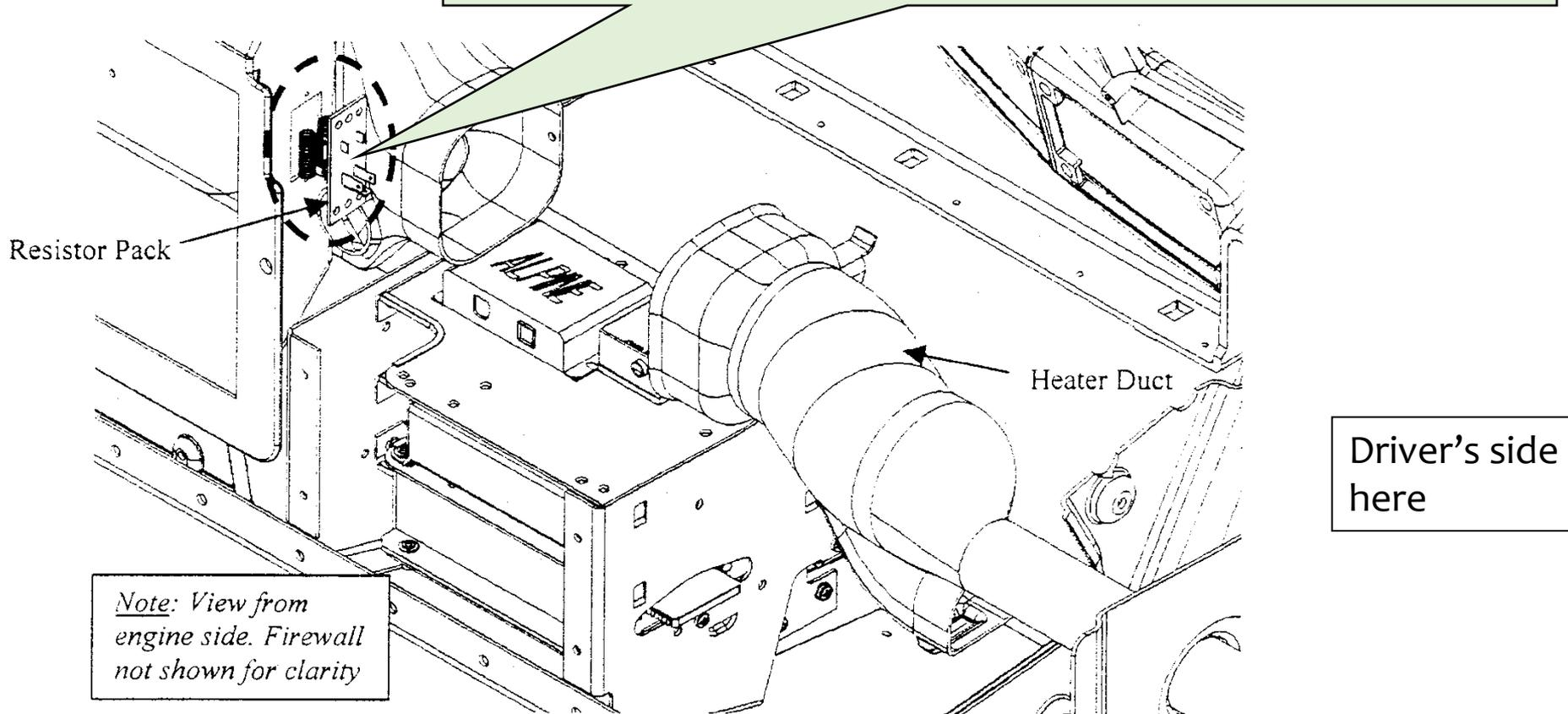
\* Must remove cup holder to get at resistor pack. Slide heater duct towards Driver's Side
