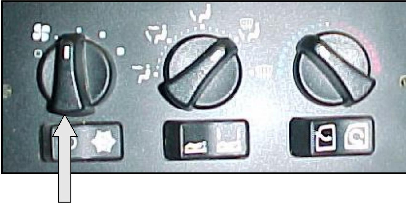
The T2000 has the cab blower circuit wired up as ground side switching and sleeper blower circuit is the opposite - power side switching.
