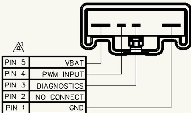
**Multi meter have negative lead in pin 1 and have the positive lead at PWM input pin 4 to check for 35hz signal**
