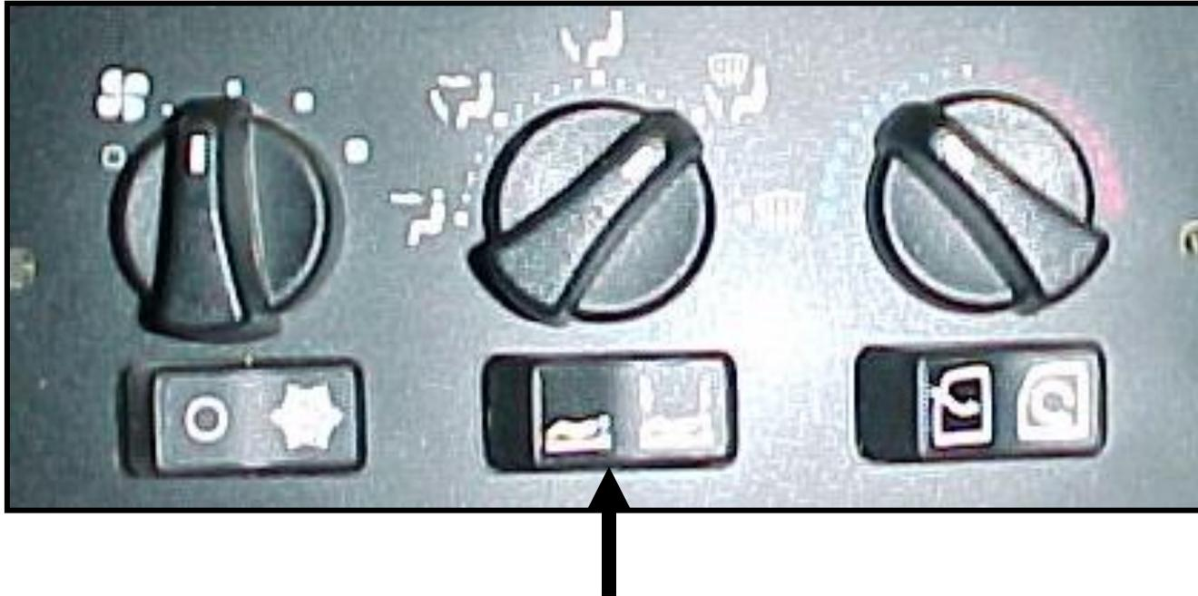
The Sleeper Rocker Switch controls power to the Sleeper Control Panel through circuit number P124SHA.
