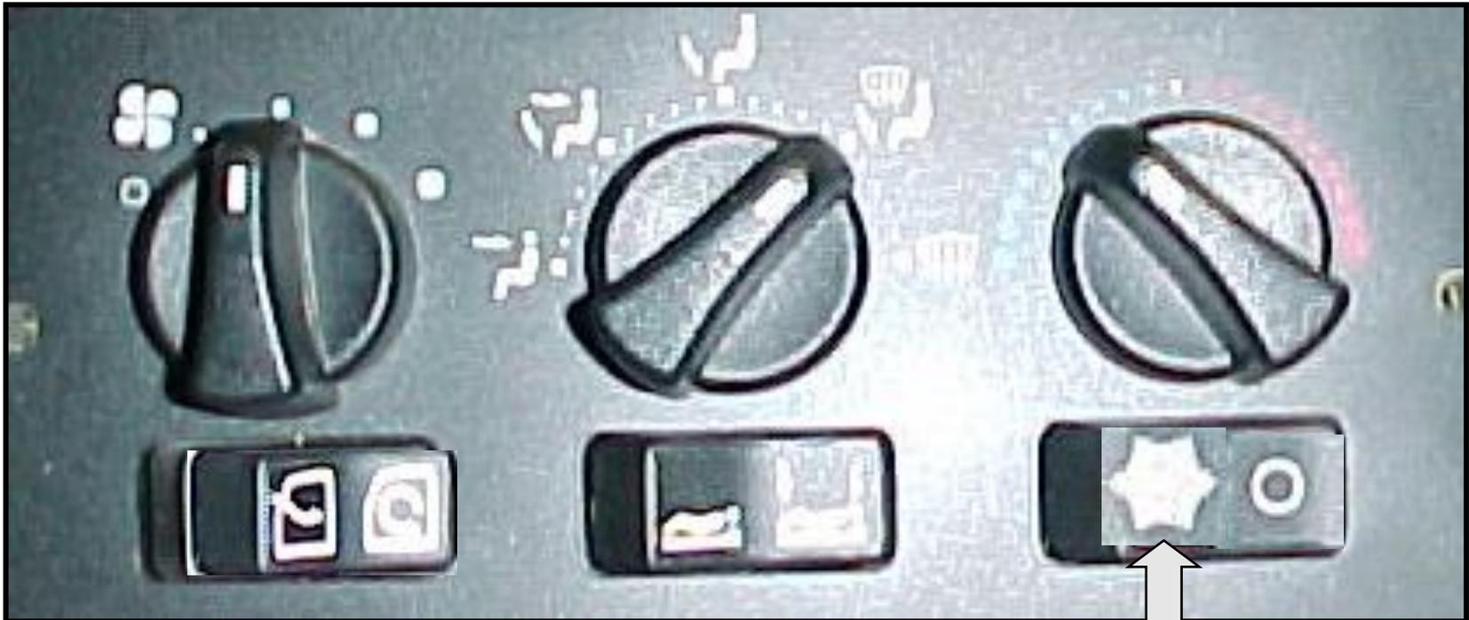
**A/C switch on the right side of the control panel**
