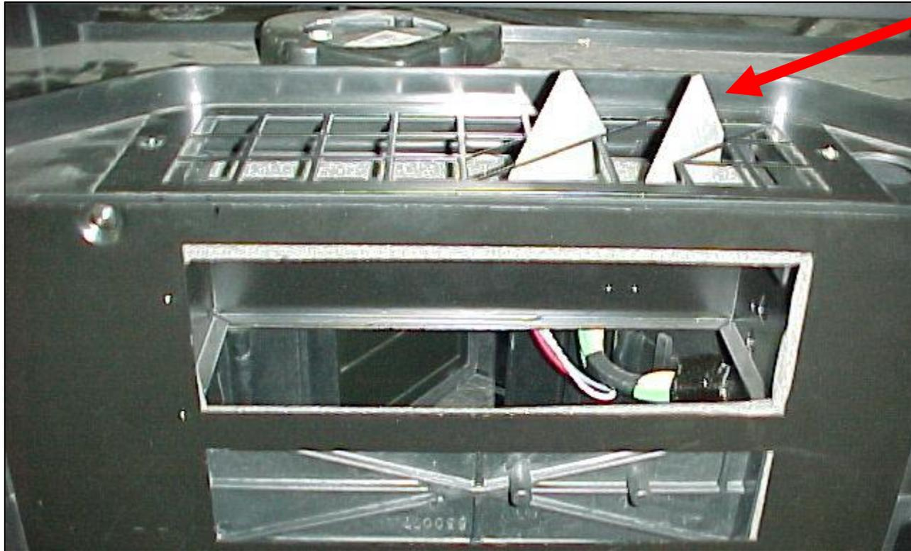
**Put unit into defrost mode before removing unit from under dash, as the tabs will be damaged during removal otherwise.**
