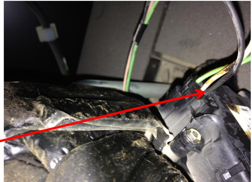
Have voltmeter in C77 SU wire and to ground, to check voltage change when blowing on Temp sensor
