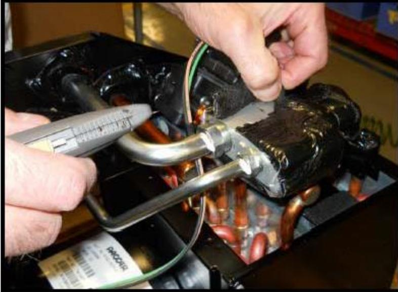
If there is no green mark, cut and peel the black insulating tape from the end of the expansion valve on the side facing UP (the end without the large round disk).
