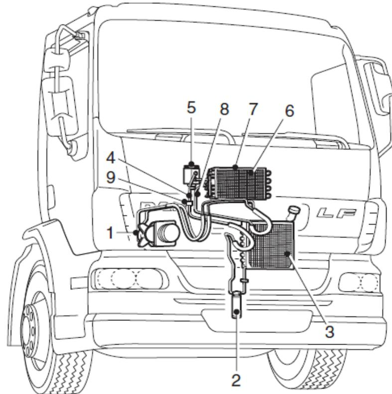
The air conditioning system is a closed system filled with R134a refrigerant. The A/C Includes a 24V Compressor.
