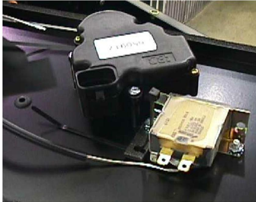
Both B-Cab and T2000 use the freeze switch in the ground side of the HVAC relay control circuit. The freeze switch *opens* at **31.5° F** and *closes* at **40° F**.
