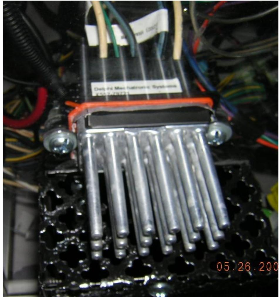
**Replaces the Resistor Block / Thermal Fuse**
