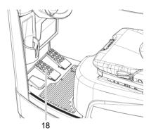
If the brake pedal is applied suddenly just before the truck stops, the drive brake also applies and is released when the brake pedal is released.
