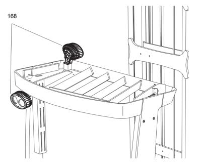
The floor spot (168) is available both in the drive direction underneath the overhead guard and in the load direction above the overhead guard.
