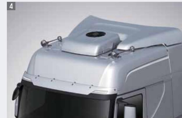
1. Application of corner vane to reduce side contamination
