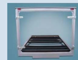
Rear door frame thickness (2.3mm → 3.2mm)
