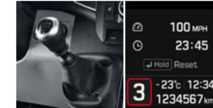
**6-speed transmission and Gear Shift Indicator (GSI)**
