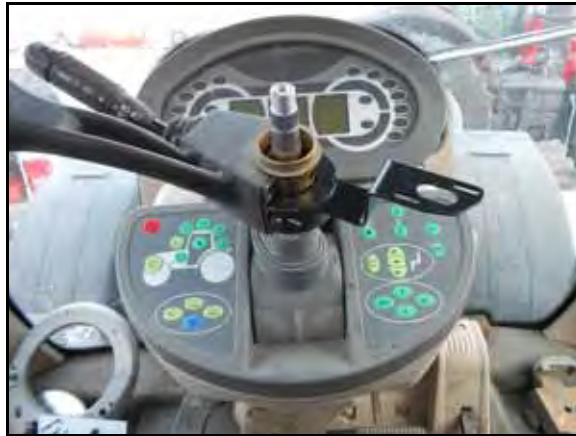
FIGURE 7. Anti-Rotation Bracket Installed
