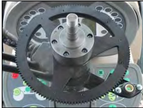
FIGURE 11. Male Spline Adapter Assembly Installed
