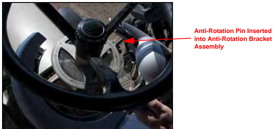
FIGURE 16. Anti-Rotation Pin Installed in Bracket Assembly
