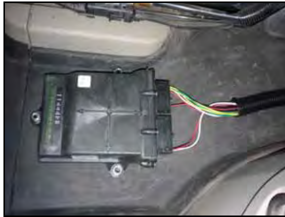
FIGURE 6. Node harness Connected to the Node
