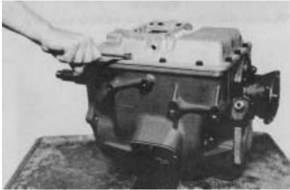
Figure 1 - Remove remote control or shift tower from control cover. Remove control cover capscrew and lock-washers
