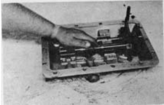
Figure 77 - Remove 1st & Reverse shift fork, rail and lug assembly.
