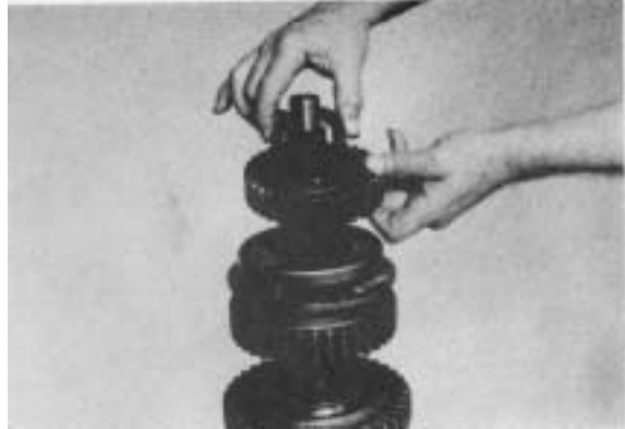
Figure 26 - Remove locating washer and 3rd gear.
