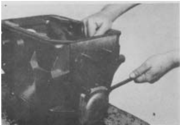
Figure 13 - Remove countershaft rear bearing cap bolts & washers.
