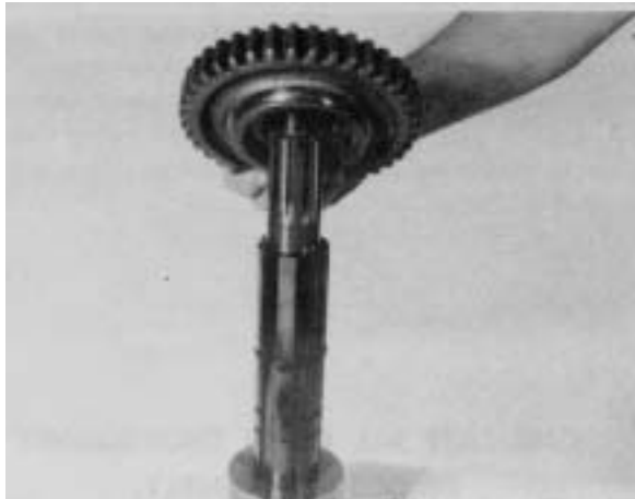
Figure 96 - Install 1st & Reverse sliding gear locating ring on mainshaft. Install sliding gear on shaft with shift fork groove as shown.
