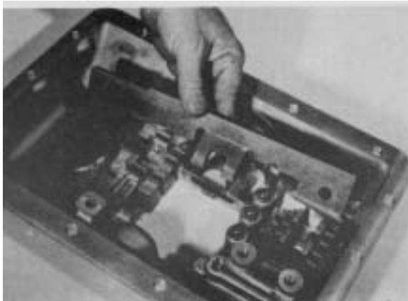
Figure 46 - Remove 1st & Reverse shift rail.
