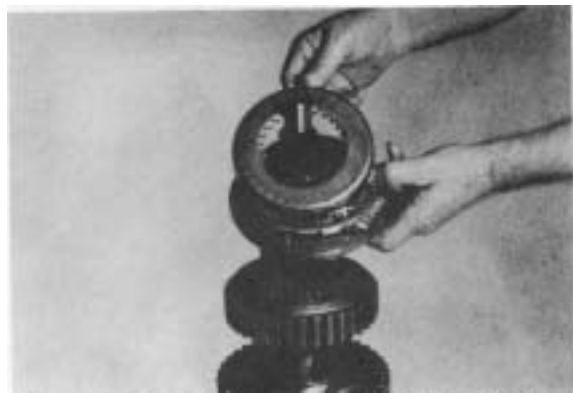
Figure 27 - Remove 2nd & 3rd synchronizer cup and synchronizer assembly.
