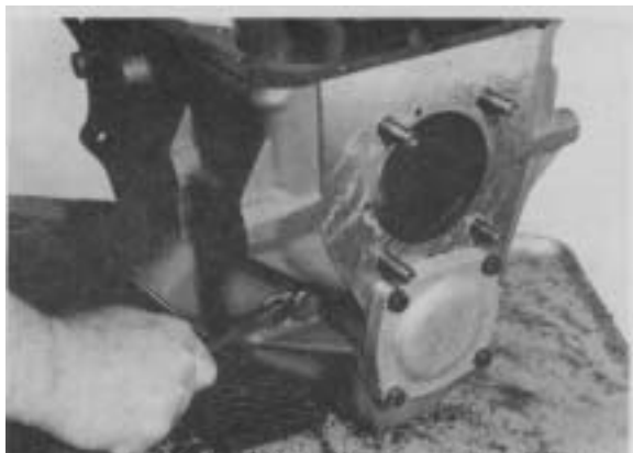
Figure 10 - Remove reverse idler shaft lock screw and lock.
