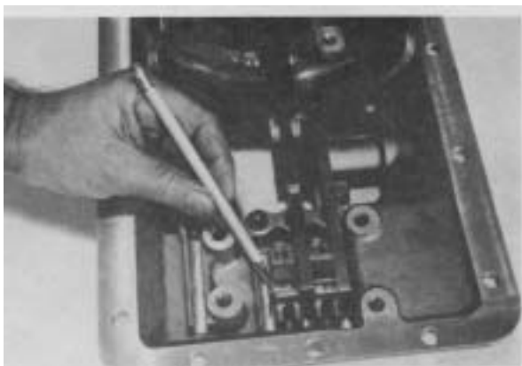
Figure 61 -Install 2nd interlock tapered pin. Align pin with interlock cross pin hole.
