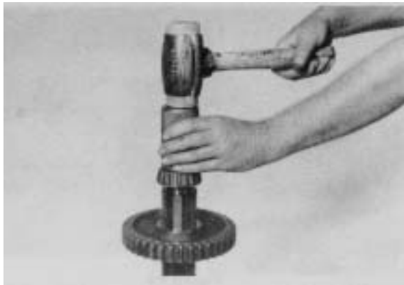
Figure 97 - Install mainshaft rear bearing with large diameter of taper toward sliding gear.
