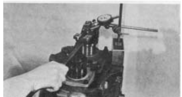
Figure 134 - Place transmission in vertical position, with main drive gear pointing down. Install transmission output flange and torque the nut. Roll main drive gear and mainshaft to seat front rear taper bearings. Position a dial indicator as shown. Pry on output flange to get mainshaft and play. End play must be between .002 - .008 [0,06 - 0,20]. Add shims for more end play or remove shims for less end play. NOTE: each time a change is made, retorque stud nuts and roll mainshaft. Apply Loctite 510 to both sides of each shim during final assembly.
