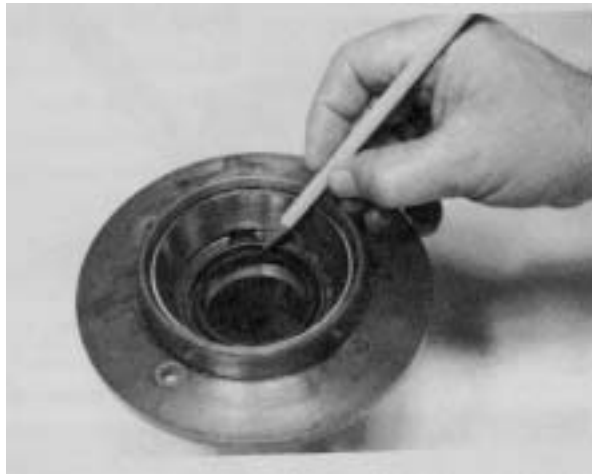
Figure 125 - Install new oil seal with lip of seal up in main drive gear bearing cap.
