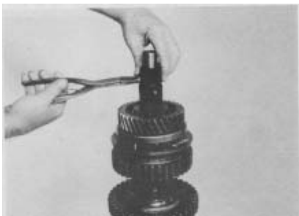
Figure 25 - Remove 3rd gear retaining ring.
