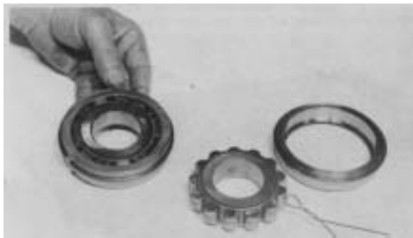
Figure 114 - Shows one bearing with all rollers held in place with a rubber band. The other bearing with the rubber band removed and rollers held in place by the outer race. Use caution when removing bearing as not to allow the rollers to slip out of cage and race
