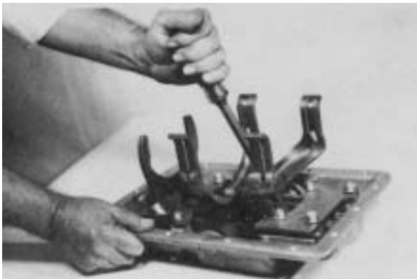
Figure 31 - Remove front rail support cap screws.
