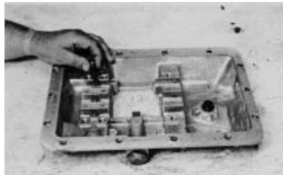
Figure 86 - Position the mesh lock spring and ball, 3 each, in spring pockets. (See cross section illustration Figure 85-A).
