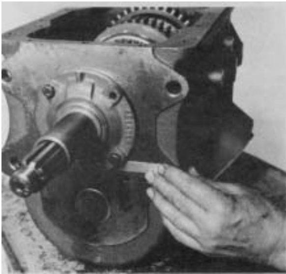
Figure 131 - Use taper gauge at other capscrew as shown. Record gap. Example: .037 [0,93 mm] average between one capscrew and the other would be .036 [0,91 mm]. Using .036 as the average gap between the bearing cap and housing, add .016 [0,40 mm]. Example: .036 + .016 will give a shim pack of .052 [1,32 mm]. This shim pack example would give a mainshaft end play of .002 to .008 [0,051 - 0,203 mm].
