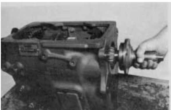
Figure 126 - Position main drive gear bearing cap on main drive gear. Lube oil groove in cap must be at the top.
