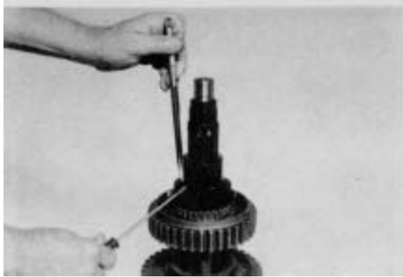
Figure 101 - Install shift hub sleeve retainer ring
