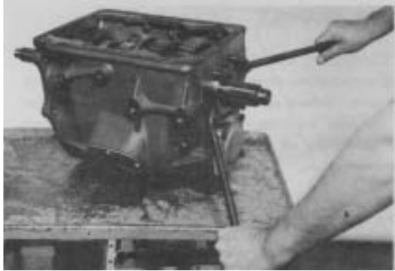
Figure 5 - Tap on input drive gear. This will move mainshaft rear bearing back far enough to be able to pry rear bearing outer race out of transmission case.
