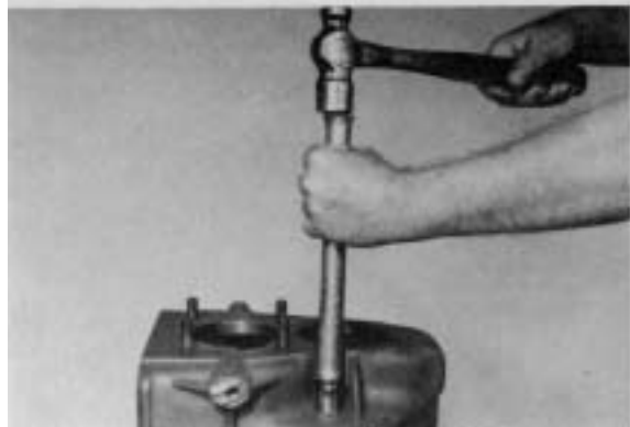
Figure 110 - Insert idler shaft through case and idler gear. NOTE: Idler shaft lock groove must line up with lock bolt hole. Drive shaft into position. Install shaft lock and bolt. Tighten bolt 20 to 25 lb. ft. torque [27,2 - 33,8 N.m].
