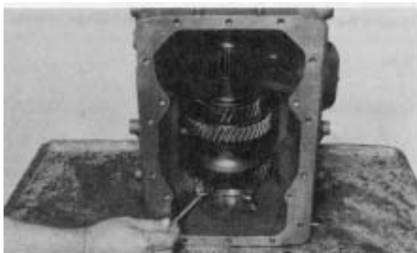
Figure 115 -Position countershaft in case as shown. Support each side of the drive gear with a 1/4" flat bar to prevent damage to the countershaft pilot bearing when installing the countershaft rear bearing. Do not disrupt countershaft pilot bearing needles.
