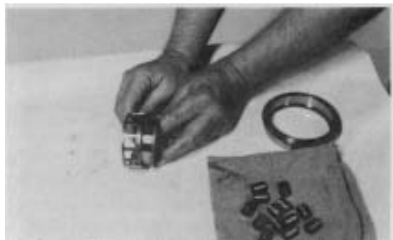
Figure 112 - Position the countershaft rear bearing inner race in the roller cage.
