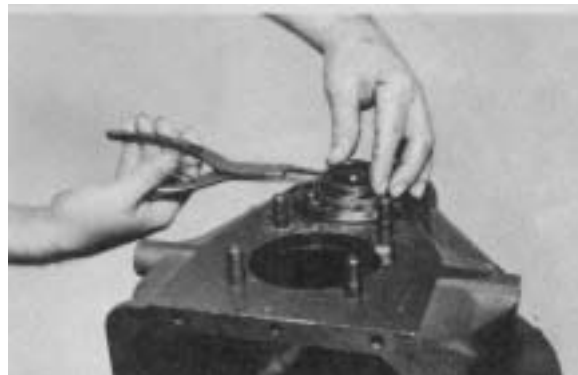
Figure 118 - Install the countershaft rear bearing retainer ring. Remove the flat bars supporting the countershaft drive gear.
