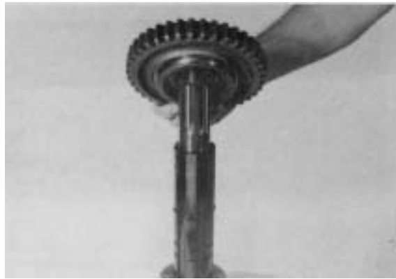
Figure 33 - Remove 1st & Reverse sliding gear.
