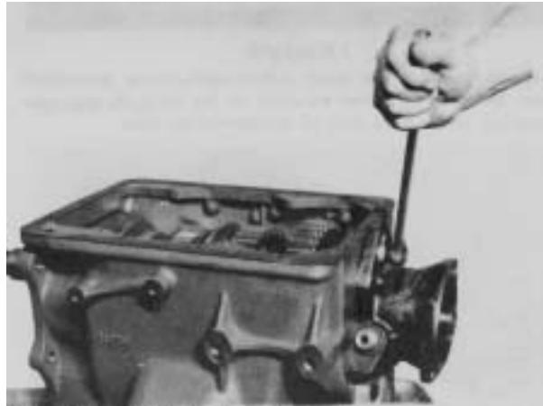
Figure 3 - Lock transmission in two gears and remove brake drum or universal joint nut. Remove mainshaft rear bearing cap bolts and washers and stud nuts and washers.
