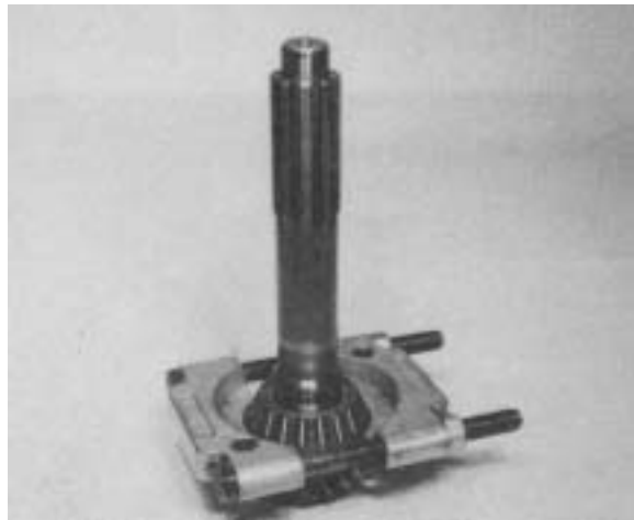
Figure 34 - If main drive gear taper bearing is to be removed, split puller shown is recommended.
