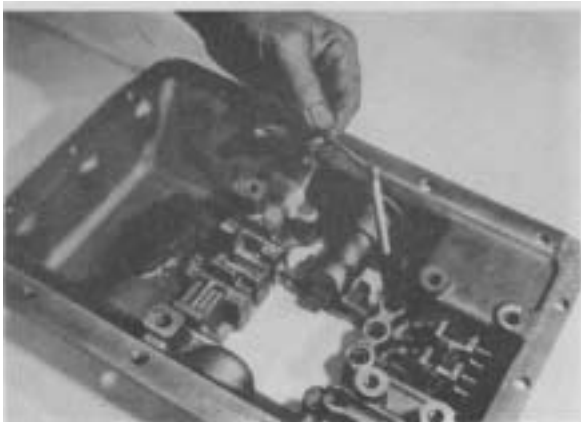
Figure 48 - Remove poppet springs, quantity 4.
