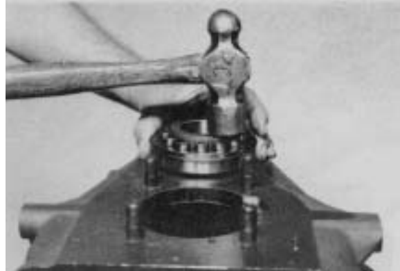
Figure 116 - Tap countershaft rear bearing inner race on countershaft until the outer race enters the case bore.
