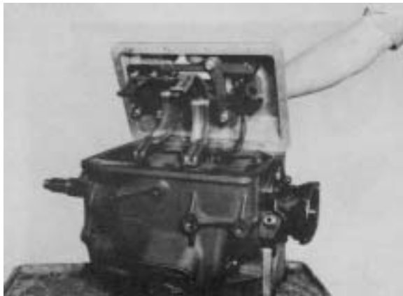
Figure 2 - Remove control cover assembly from transmission.
