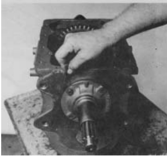
Figure 130 - Using a taper gauge at a capscrew, as shown, record gap between bearing cap and housing. Example: .035 [0,88 mm].
