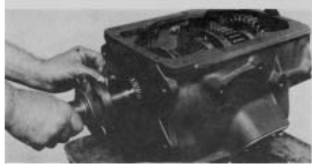
Figure 132 - Using example .035 - .037 - average .036+.016 .052 shim pack, position shim pack and main drive gear bearing cap on main drive gear. Lube oil groove in bearing cap must be at the top.
