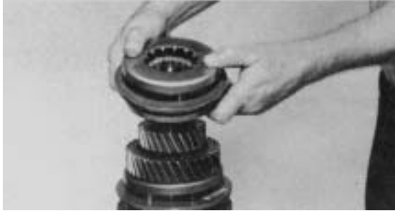
Figure 107 - Install the 4th & 5th speed synchronizer and synchronizer cups on shift hub sleeve.
