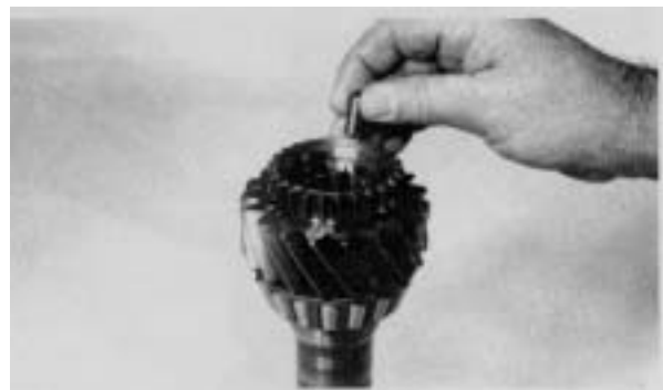
Figure 94 - Press new taper bearing on drive gear. Turn gear over. Using a high quality heavy grease, coat roller bearing surface. Place rollers in grease as shown.
