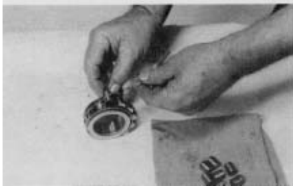
Figure 113 - A rubber band was used to hold the rollers in place in the bearing cage.
