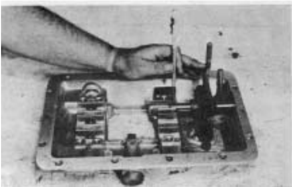
Figure 78 - Using a small magnet remove the 1st & Reverse shift fork rod lock pin.
