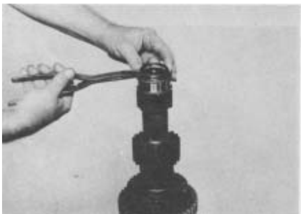
Figure 19 - If countershaft rear bearing is being replaced, remove outer race retainer ring.
