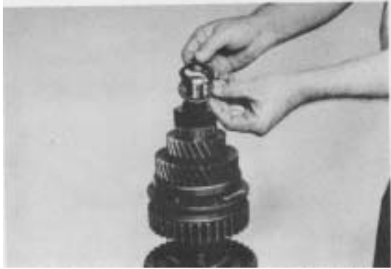
Figure 23 - Remove shift hub bearing race and bearing.
