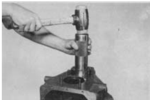
Figure 117 - Use a driver that will fit over the end of the countershaft but not larger than the bearing inner race. Tap the outer race in the bearing bore and drive the inner race on the countershaft.
