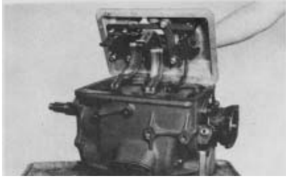
Figure 71 - With new gasket in position and with transmission in neutral, position control cover over gears aligning shift forks in shift cover with gear shift hubs. If control cover is in neutral and transmission is in neutral, transmission drive gear should turn without output shaft turning.
