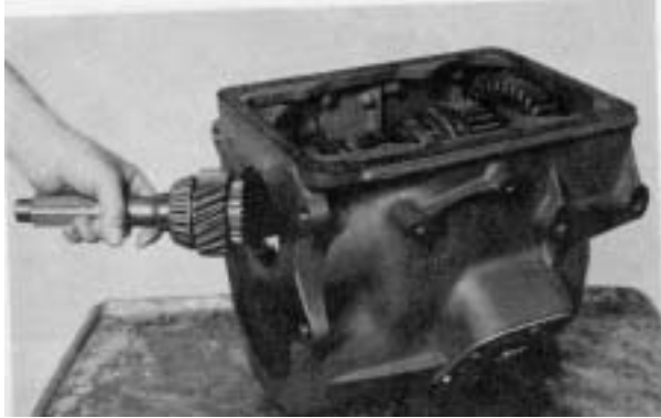
Figure 124 - With main drive gear needle rollers in place and greased, position main drive gear in housing bore. Align clutching teeth on main drive gear with teeth in 5th speed synchronizer cup.
