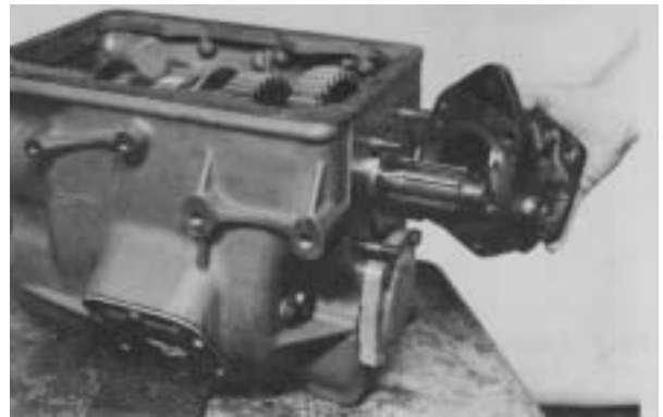
Figure 123 - Position new gasket on mainshaft rear bearing cap. Install bearing cap on studs. Install stud nut lockwashers and stud nuts. Tighten stud nuts 60 to 70 lb. ft. torque [81,4 - 94,9 N.m].
