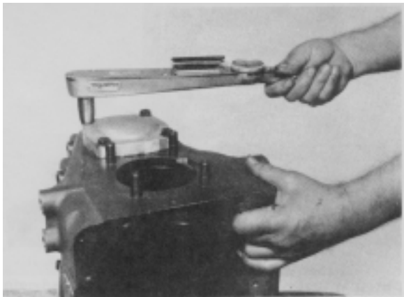
Figure 120 - Install rear bearing capscrews and washers. Tighten 20 to 25 lb. ft. torque [27,2 - 33,8N.m].
