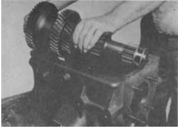
Figure 17 - Remove countershaft assembly from case.
