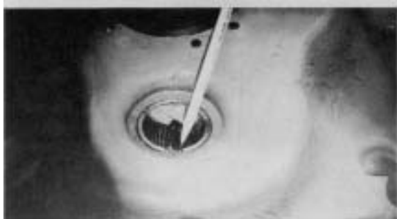
Figure 111 - Coat countershaft pilot bearing needle rollers with heavy grease to hold in place until countershaft is installed.
