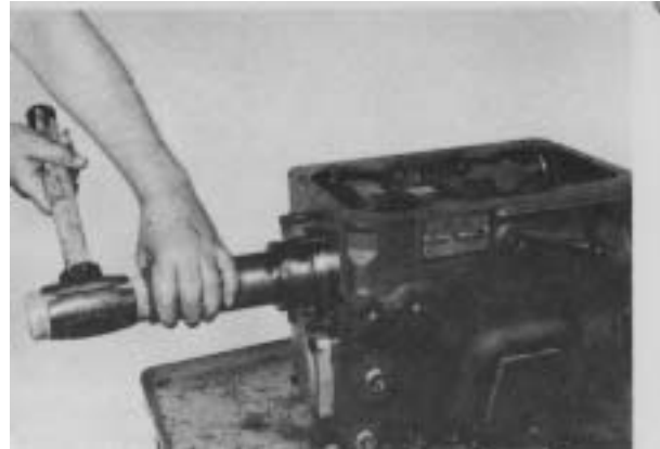
Figure 122 - Install mainshaft rear bearing cup
