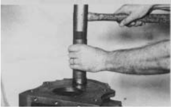
Figure 108 - If countershaft front bearing is to be replaced, remove clutch housing and drive front bearing from transmission case. Apply a light coat of Loctite 510 on the outer diameter of the new bearing. Install in transmission case as shown with end of bearing .001 to .007 below the front surface of case.
