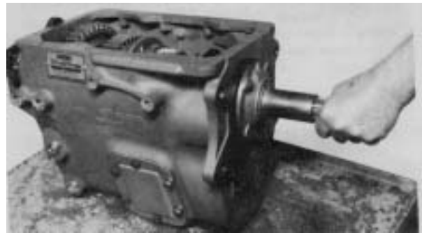
Figure 128 - Turn main drive gear and mainshaft by hand back and forth to seat taper bearings.
