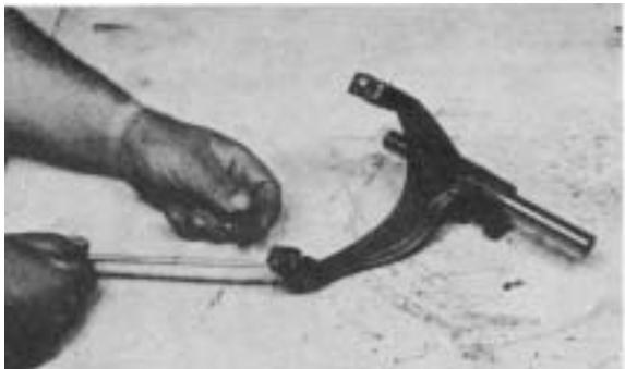
Figure 82 - Remove mesh lock spring and lock ball, 3 each. Remove crossover interlock balls, 4 each.
