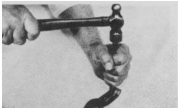
Figure 52 - If fork bushings are worn, secure fork in a vise equipped with soft jaws and remove worn bushings with a drift. Install new bushings in fork. Turn fork over on anvil of vise and secure bushing in fork using a prick punch and upsetting bushing metal on outside of fork.
