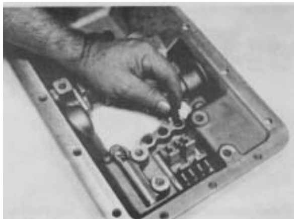
Figure 55 - Install poppet springs, quantity 4.
