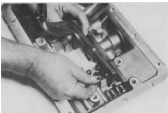
Figure 60 - Position 2nd & 3rd shift rail on poppet ball in neutral position with interlock pin aligned with 1st interlock tapered pin.
