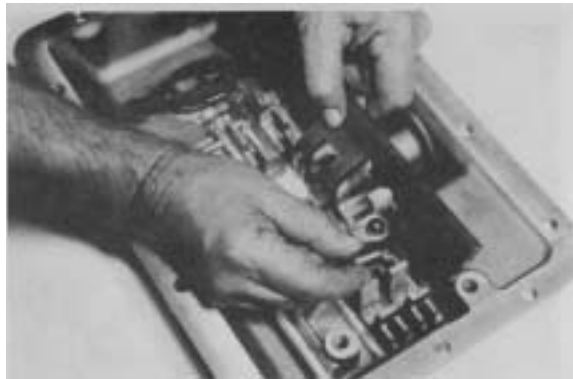
Figure 57 - Align one tapered interlock cross pin with hole in 1st & Reverse shift rail. Position rail on poppet ball with rail in neutral position.
