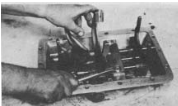
Figure 73 -Remove front and rear rail support cap-screws.
