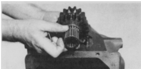
Figure 109 - Turn transmission case over. Use a heavy grease to hold the reverse idler gear thrust washers in place on idler shaft boss. Insert the 2 idler spigot bearings in the idler gear. Position idler gear between thrust washers. NOTE: Small end of idler gear to be up or toward the rear of the transmission case.
