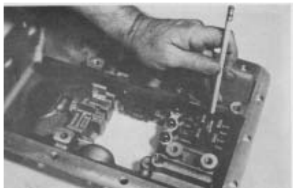
Figure 58 - Note position of tapered interlock cross pin in relation to rail.
