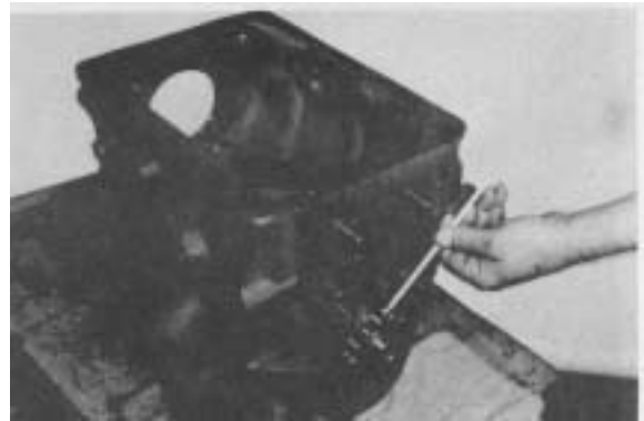
Figure 14 - Remove countershaft rear bearing cap and bearing spacer ring.
