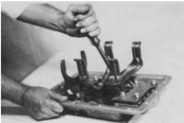
Figure 36 - With control cover in neutral, pry 4th & 5th shift to 4th speed position (toward the rear of cover).
