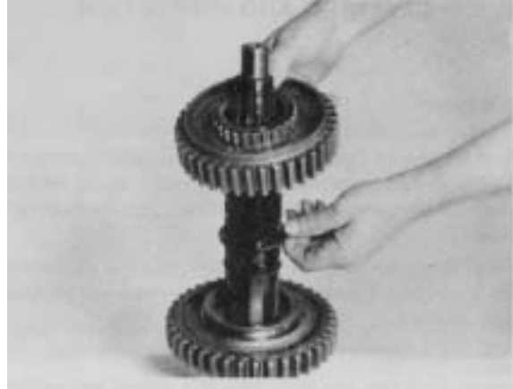
Figure 98 - Turn shaft over. Install 2nd speed locating washers and 2nd speed gear on shaft. Note clutching teeth on gear are up.
