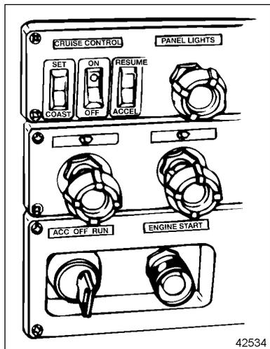
Figure 6 Typical Cruise Control Switches
