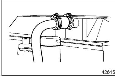
**Figure 19 Internal (in Rocker Cover) Breather Location**
