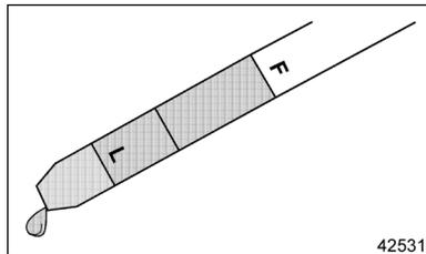
**Figure 4 Check Lube Oil Level Before Starting**
