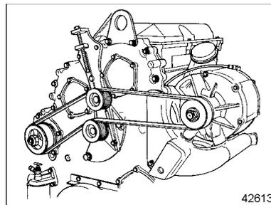
**Figure 15 Manual Tensioner Assembly with 50 DN Alternator**
