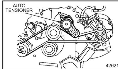
**Figure 14 Auto Belt Tensioner Assembly with 50 DN Alternator**
