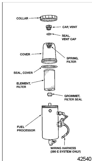
**Figure 25 Fuel Pro 382E Fuel Processor Assembly**
