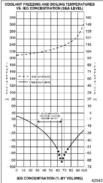
**Figure 26 Coolant Temperatures vs. IEG Concentration (Sea Level)**
