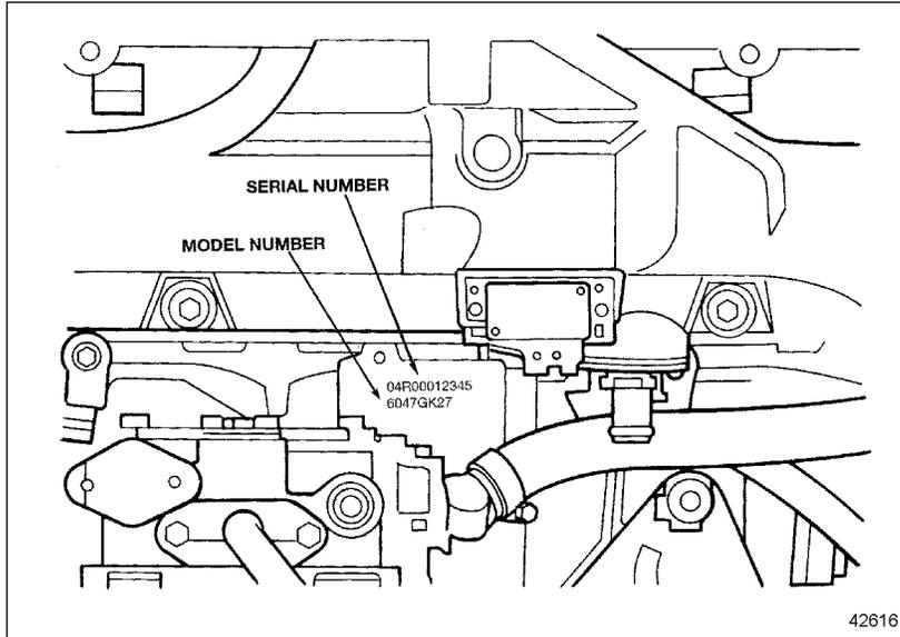
Figure 1 Location of Engine Serial and Model Numbers
