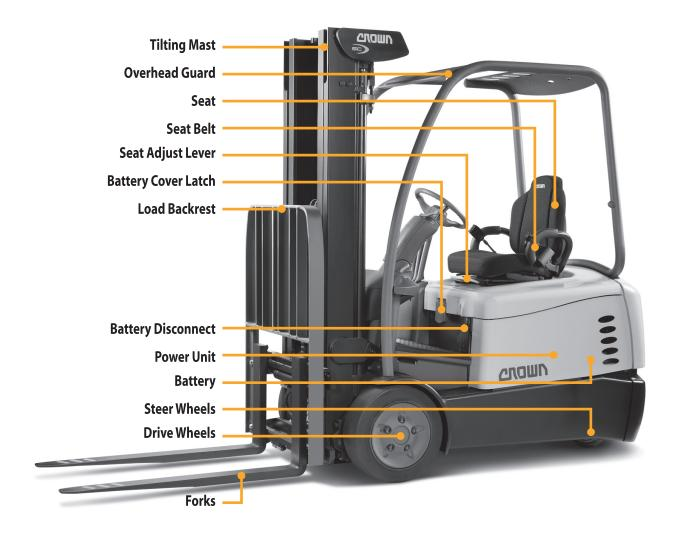
9 Lift Truck Parts Lift Truck Parts 10
