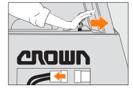
Push the Power Disconnect in the direction of the forks to disconnect the battery and cut all power.
