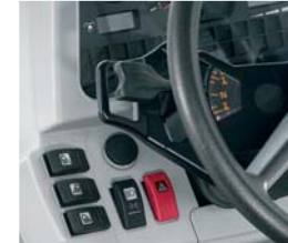
3. POWER CONTROL LEVER FOR USE WITH AUTOPOWER IV (OPTION NOT PICTURED ON PAGE 4)
