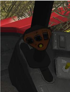
Figure 1: The hydrostatic handle
